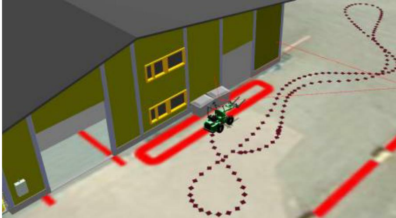
Figure 18. An example of the drive path visualisation in the simulator environment.
