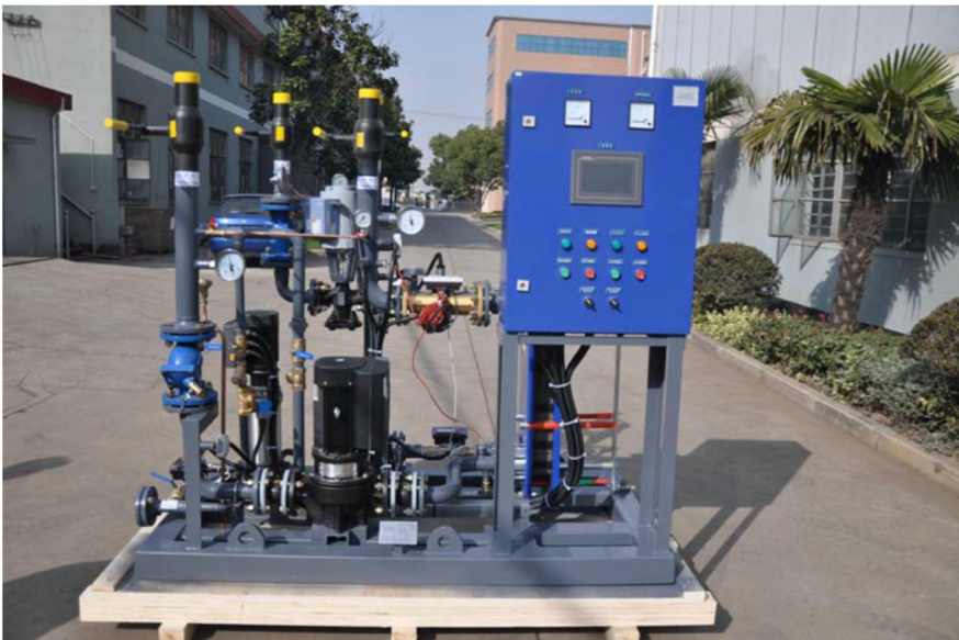
Figure 5. Small buildings heat exchanger unit.
