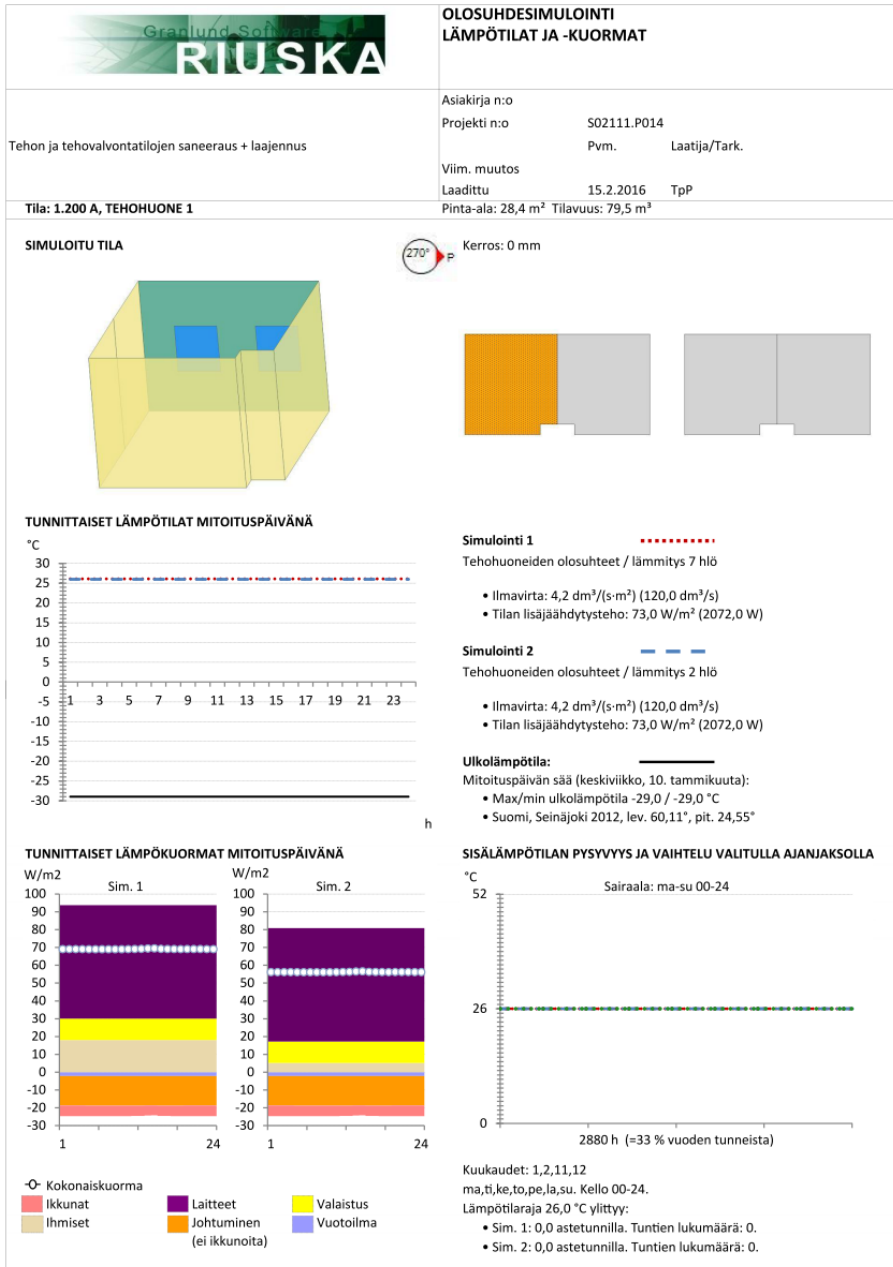
Figure 55. Heating simulation with Granlund's RIUSKA software.
