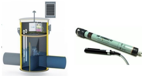
Figure 10. On the left, EHP-Monitoring Station for water flow and quality monitoring in arctic field conditions can measure several parameters online, such as water flow/level, pH, EC, Eh, DO, NO 3 -N, NH 4 -N, T, COD, TOC, solids, and turbidity. On the right, a portable water level and quality monitoring device for wireless monitoring of groundwater and surface water level and quality in the field. Depending
