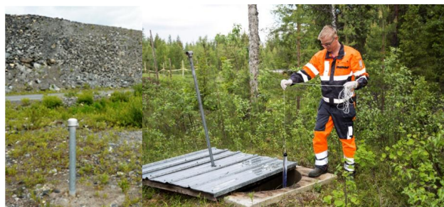
Figure 8. a) Groundwater observation well. b) Taking a groundwater sample from private domestic well. (Photos: (a) Tiina Kaipainen, GTK and (b) GTK.)
