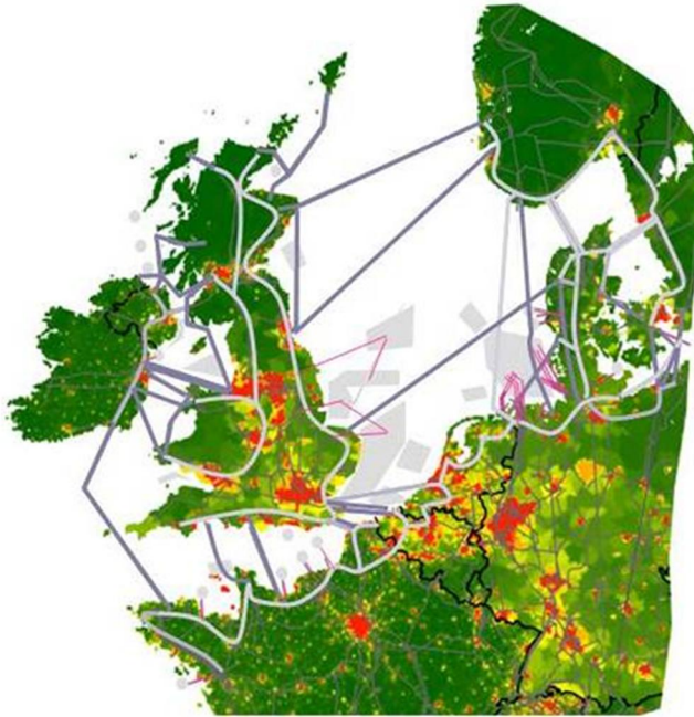
Figure 21. North Seas Offshore Grid Infrastructure 2030 according to ENTSO-E's European Ten Year Network Development Plan TYNDP (ENTSO-E, 2014). (Light grey: existing connections, dark grey: new connections, grey areas: wind exploitation areas.)
