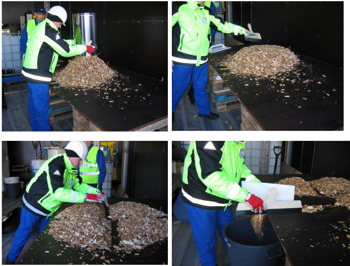
Figure 3.8. Division of a sample using the coning and quartering method. Figure and photos: Eija Alakangas, VTT.
