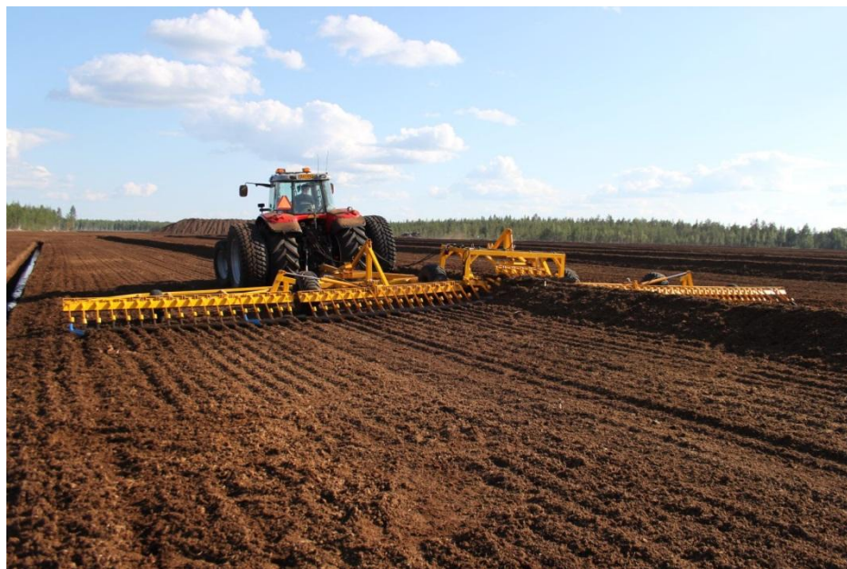
Figure 6.2. Harrowing of milled peat. Figure: Vapo Oy.
