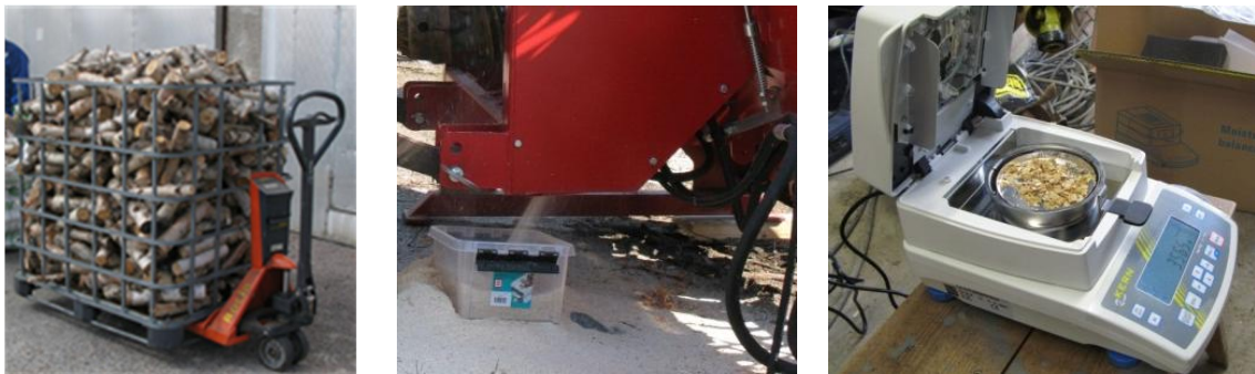
Figure 2.3. Determination of moisture content from a smallwood unit using sawdust. Photos: VTT.
