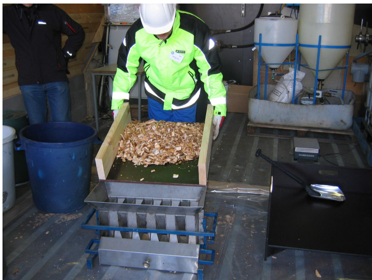
Figure 3.7. Division of a wood chip sample using a riffle box. Photo: Eija Alakangas, VTT.
