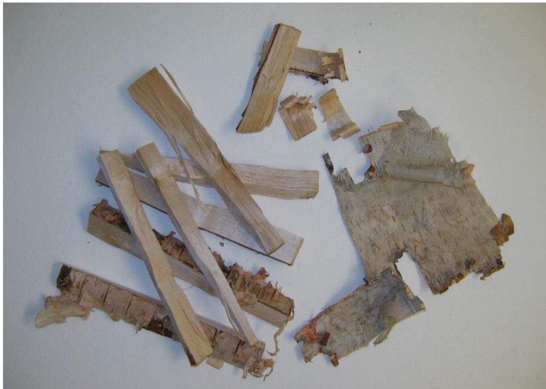
Figure 4.16. Kindling. Wood used as kindling has a diameter of approximately 2 cm. Figure: Eija Alakangas, VTT.
