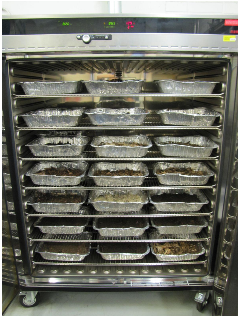
Figure 2.2. Determination of the moisture content of fuel. Photo: Labtium Oy.
