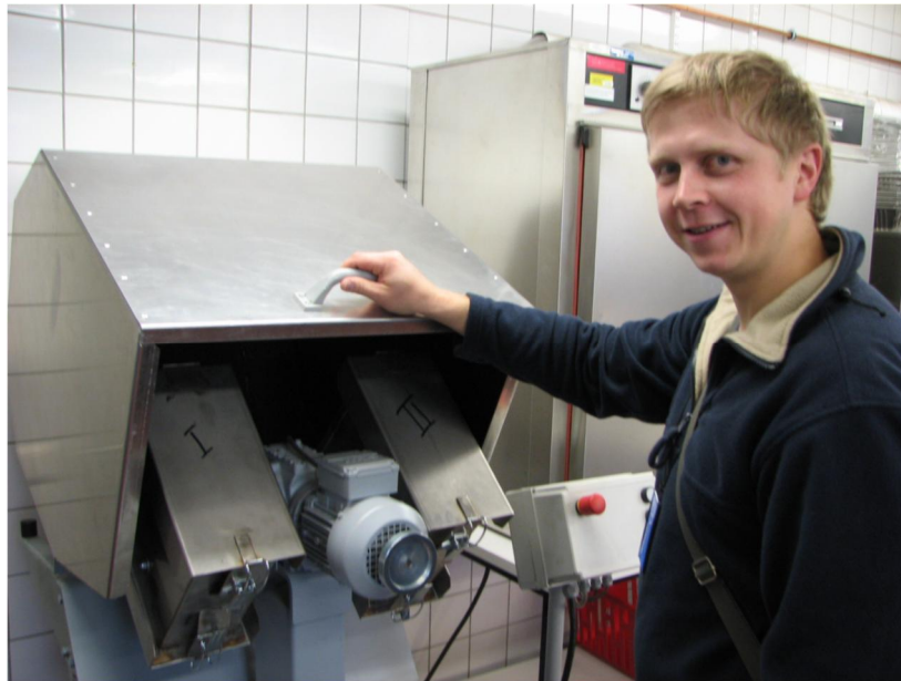
Figure 2.6. Tester for the mechanical durability of pellets. The device consists of two drums. Photo: Labtium Oy.
