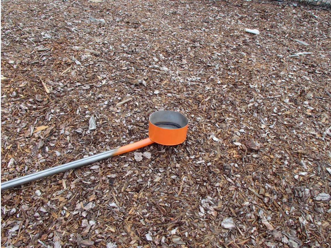
Figure 3.2. A three-litre sampling scoop with a long handle, which is ideal for forest chip sampling. Photo: Ismo Tiihonen.
