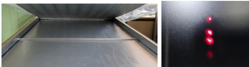
Figure 3.26. Prototype 4 rear insulation assembly: 30 mm low-e foil cladded PIR-foam and 20 mm air gap.
