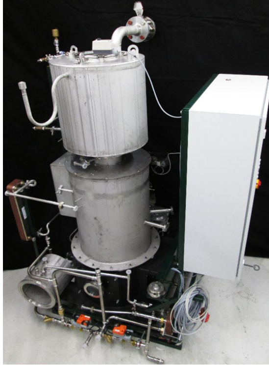
Figure 3.34. Uninsulated second stage of a biomass driven absorption machine including piping of mixing circuit and control cabinet.
