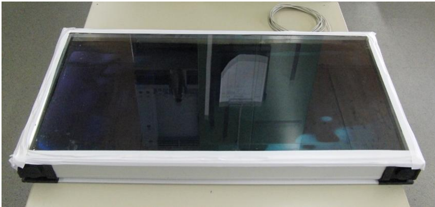
Figure 3.16. Prototype 0: Quarter-scale model for foil straining tests.
