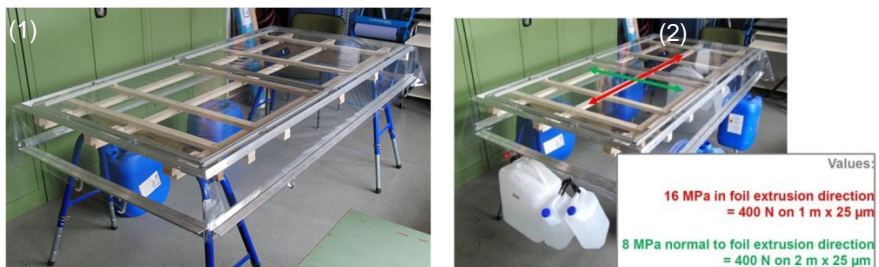
Figure 3.11. ETFE foil on second frame ready for straining (1) and after (2).
