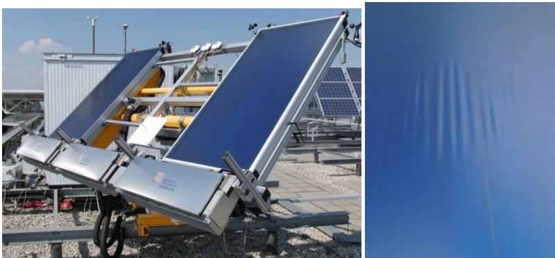
Figure 3.18. Prototype 1 on ZAE Bayern outdoor test-rig (right) and reference collector SF100-03 series type (left). Prototype 1 shows small wrinkles in the middle of the aperture area at 110 °C fluid mean temperature.
