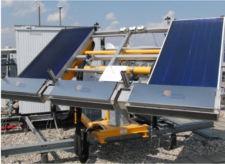
Figure 3.21. Prototype 2 (right) and series SF100-03 reference collector (left) on ZAE test-rig.
