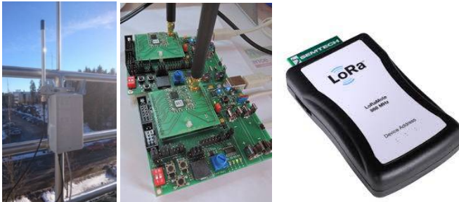
Figure 2. Various LoRa off-the-shelf gateway and node development kit components.
