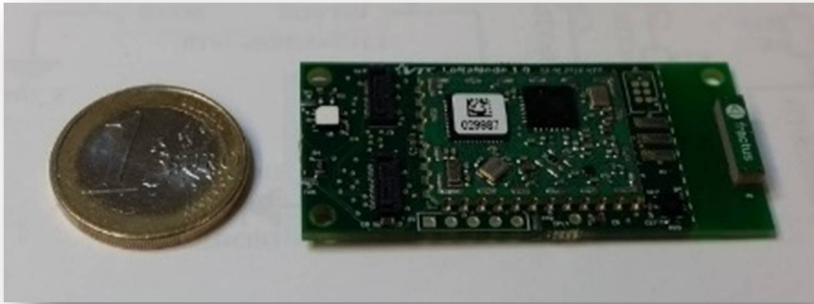
Figure 5. VTT LoRa node circuit board developed and demonstrated in a module project.
