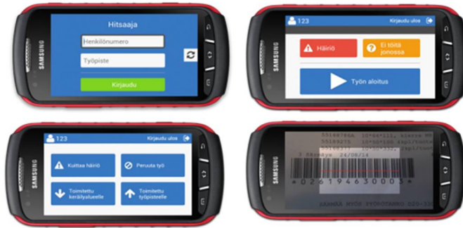
Figure 2. User interfaces of a mobile welding job reporting and control (source: Suomen Levyprofiili Oy).
