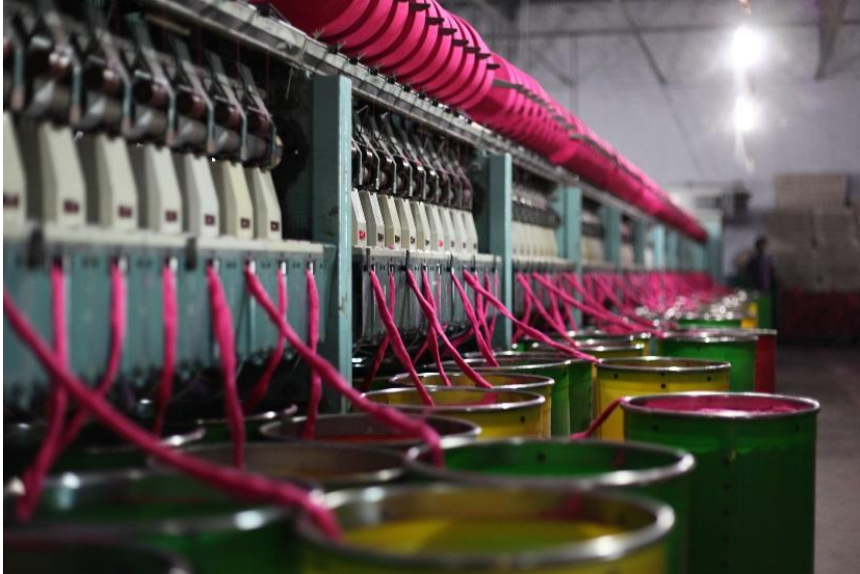
Figure 22. Spinning of mechanically recycled fibres at Pure Waste Textile's Tirupur Factory.
