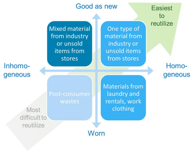
Figure 16. Raw material sources for reutilization in textile applications based on homogeneity and wear of materials.
