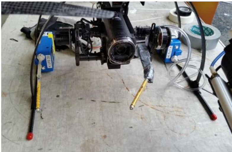
Figure 105. Two Gilian LFS-113DC low flow samplers with detection tubes for ammonium, mounted in the Videodrone X8. (Image: VTT/Jukka Sassi)
