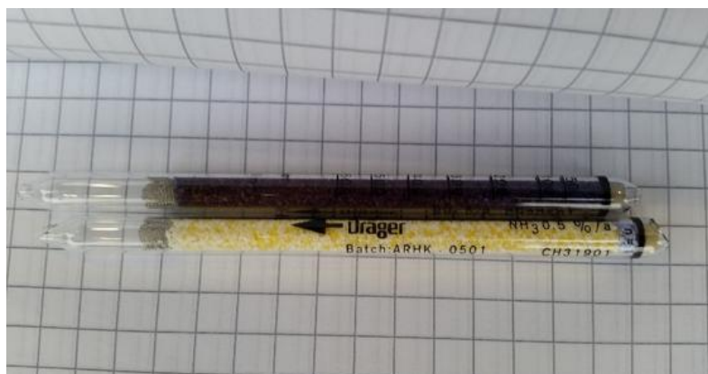
Figure 96. Two Dräger indicator tubes for NH 3 , used (above) and unused (below). (Image: VTT/Jukka Sassi)
