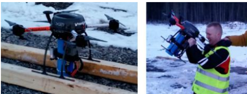
Figure 64. BlueHawk sensor installed on UAS but operated as a handheld set-up due to excess payload. (Images: VTT/Jukka Sassi)
