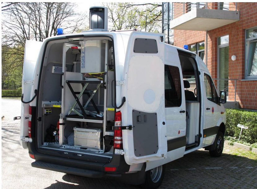
Figure 31. SIGIS 2-system mounted in an emergency vehicle in Germany. (Bruker, 2017)
