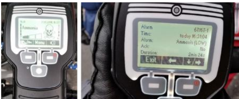
Figure 112. The ChemPro100i clearly detected ammonium. (Images: VTT/Jukka Sassi)
