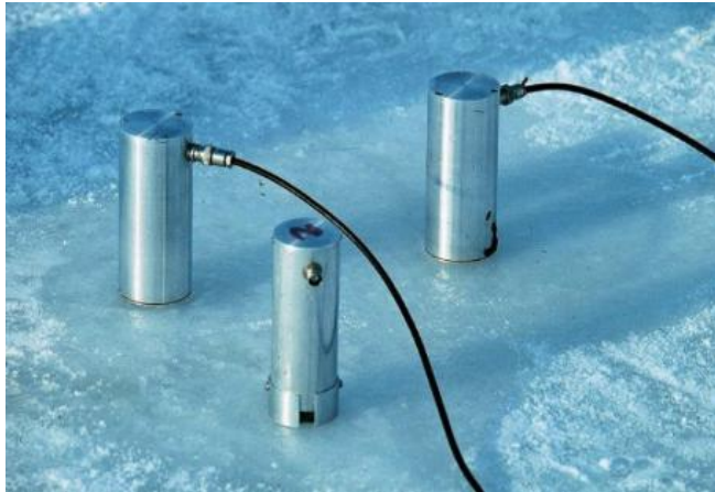
Figure 25. Acoustic transducers placed on sea ice for a field test to detect oil under ice. (Fingas and Brown, 2013)
