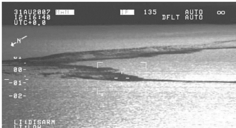
Figure 15. Example of FLIR image of an oil spill. (Puestow et al, 2013)
