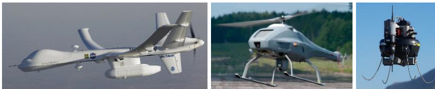
Figure 39. Examples of UAVs: the Altair by General Atomics Aeronautical Systems Inc. (left), Skeldar V-200 by Saab Aerospace (middle), and the T-Hawk™ Micro Air Vehicle from Honeywell (right).
