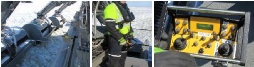
Figure 34. Heavy duty ice brushes in operation during the Kemi Arctic 2015 exercise. (Images: VTT/Jukka Sassi)
