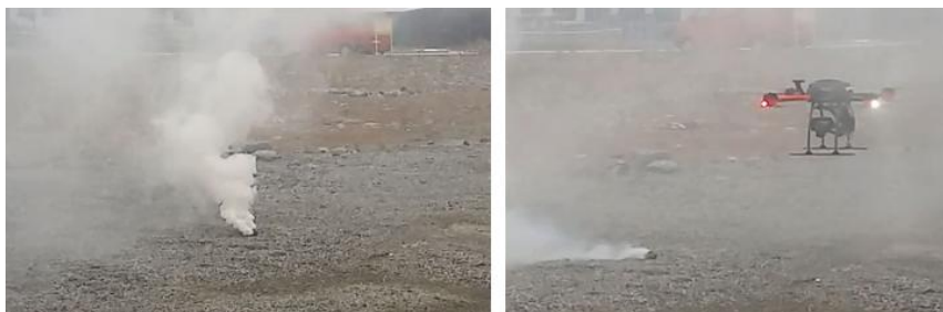
Figure 111. The turbulence effect caused by the drone. (Image: VTT/Jukka Sassi)
