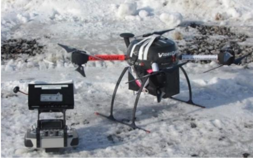
Figure 65. The hyperspectral camera by Rikola Ltd installed in the UAS on Day 2. (Image: VTT/Jukka Sassi)
