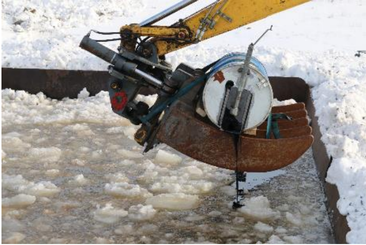
Figure 55. The 200 l oil barrel of HFO180 with a release lid in the bucket of an excavator. (Image: SYKE/Jouko Pirttijärvi)
