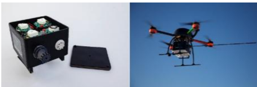
Figure 95. Aeromon BH-8 module with its lid open (left) and mounted on a drone (right). (Aeromon, 2016)
