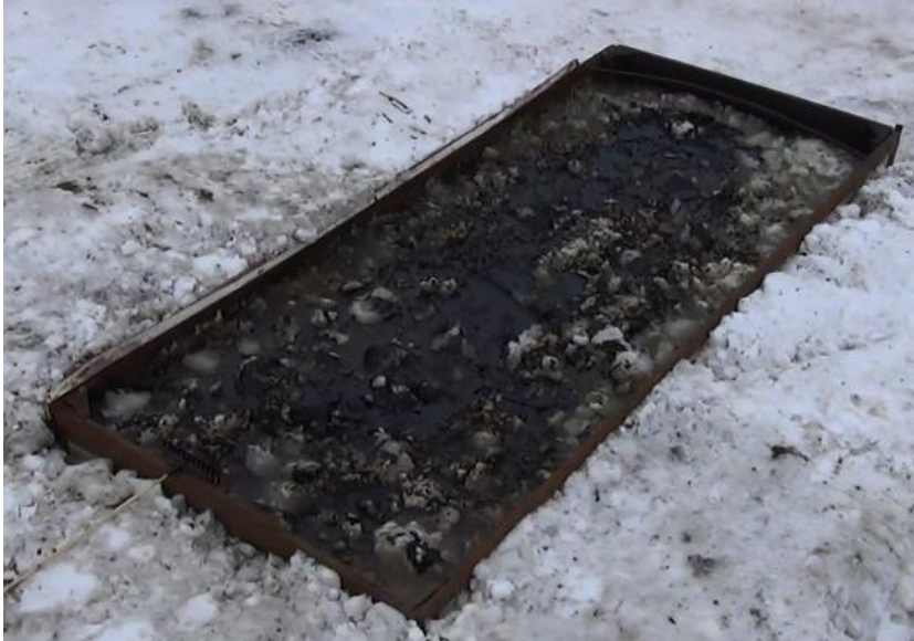
Figure 57. Aerial view of basin C with 50 l of oil on ice and on water. (Extracted from the video by AIF)
