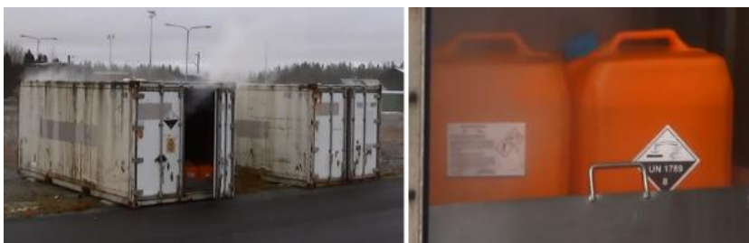
Figure 114. Extractions from the AIF video of Videodrone X8 drone during the identification of acid containers inside the container. UN 1789 8 stands for hydrochloric acid (HCl).
