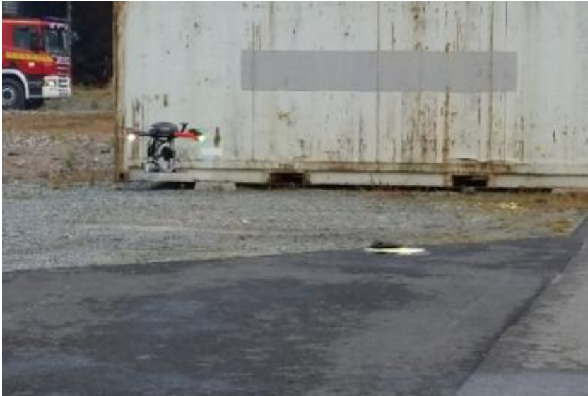
Figure 107. The drone flying near the cloth with HCl. (Image: VTT/Jukka Sassi)
