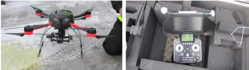
Figure 60. The UAS used in the test trials with the video camera mounted, and the remote control console with the video controls. (Images: VTT/Jukka Sassi)
