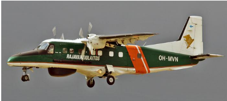
Figure 36. Dornier 228 equipped with Side-Looking Airborne Radar (SLAR) and IR/UV scanner. (Image: The Finnish Border Guard)
