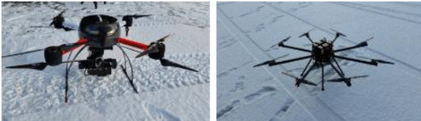
Figure 91. Videodrone X8 (left) with video and FLIR cameras mounted, and Airborne KX8 (right) with a weight of 3.5 kg to imitate a sensor payload. (Images: VTT/Jukka Sassi)
