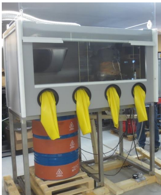
Figure P4: The evaporation and waste treatment box during assembly work.
