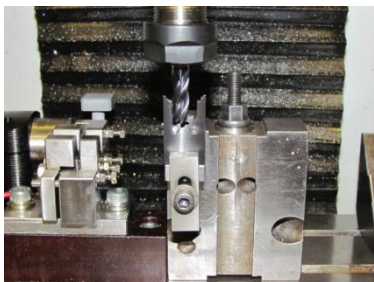
Figure 50: Separation of the CT sample from the pressure tube fragment
