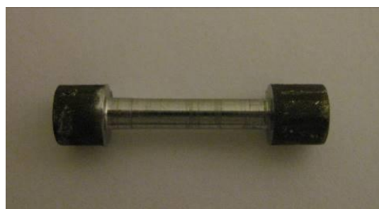
Figure P13: A round bar cut from a half of the tested Charpy specimen (a), a tension specimen machined from the round bar (b)
