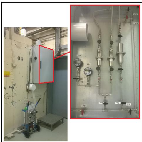
Figure P37: Valves system for gas sampling Use the Caption style and label Figure
