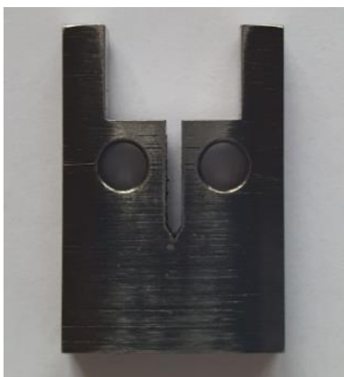
Figure 53: CT sample manufactured out of non-irradiated CANDU pressure tube
