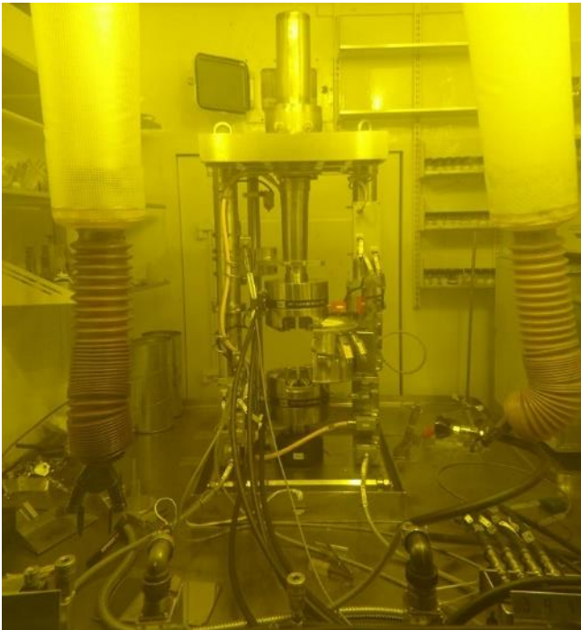
Figure 64: In cell 120 kN tensile tester (left) and industrial remote control of the power manipulator.
