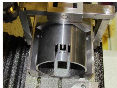
Figure 50: Separation of the CT sample from the pressure tube fragment
