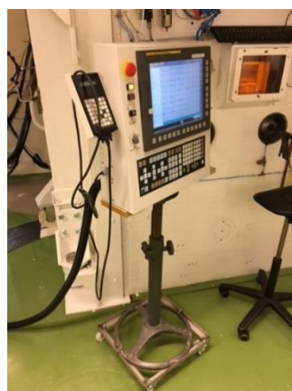
Figure P11: A new 7-inch door was fitted to the hot cell (left). Operator control panel of the installed EDM (center). A steerable in-cell IP-camera helps the operator to see all corners of the cell.
