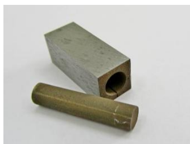
Figure P13: A round bar cut from a half of the tested Charpy specimen (a), a tension specimen machined from the round bar (b)
