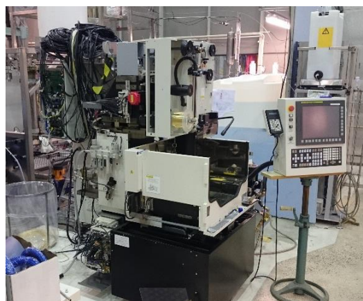
Figure P10: In-cell filters for EDM-fluid (left) and EDM under modification (right)
