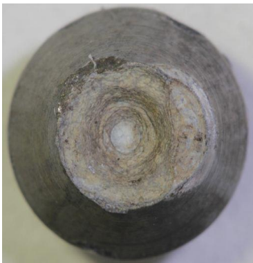
Figure 21: Hole welding failure
