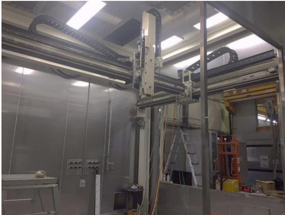
Figure 8. Precise gantry system driving by linear motor.
