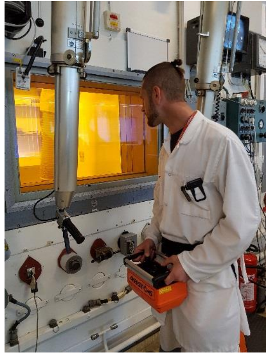
Figure 64: In cell 120 kN tensile tester (left) and industrial remote control of the power manipulator.
