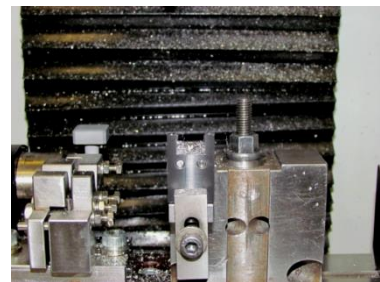
Figure 50: Separation of the CT sample from the pressure tube fragment
