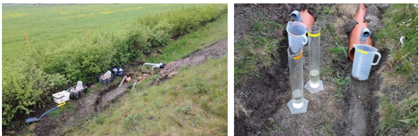
Figure A5. Data gathering in progress in June 8, 2017. 3-litre cans were used for quality sample gathering, and 1000-ml measuring glasses for manual flow rate measurements. (Images by Eero Assmuth)
