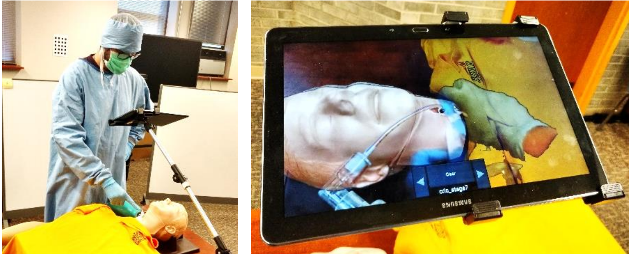
Figure 1. Left: A mentee views the operating field of a patient simulator through our tablet-based AR system. Right: View of operating field with visual annotations (virtual hand) superimposed.
