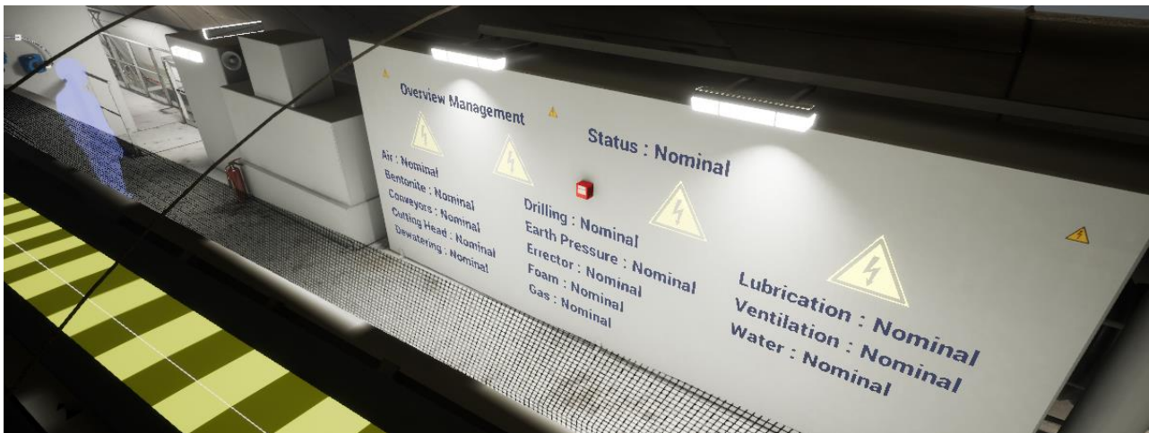
Figure 5. The main overview for supervisors working on the TBM stating the main system statuses.
