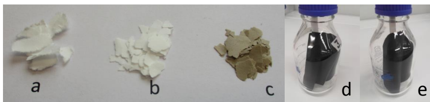
Figure 5. Cellulosic samples before and after degradation with gaseous HCl. a) Untreated Whatman 1 paper, b) Whatman 1 paper after 1.5 h treatment time with 100 kPa HCl pressure, c) Whatman 1 paper after 68 h treatment time with 100 kPa HCl pressure, d) Whatman 1 with 10 w-% water content after 72 h treatment, e) Whatman 1 with 20-% water content after 72 h treatment.
