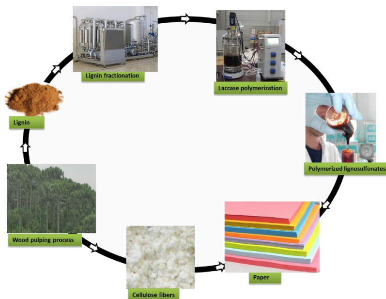
Figure 1. General overview of the scheme showing circular bioeconomy concept using lignin from the pulping process as a raw material in paper coating formulation.
