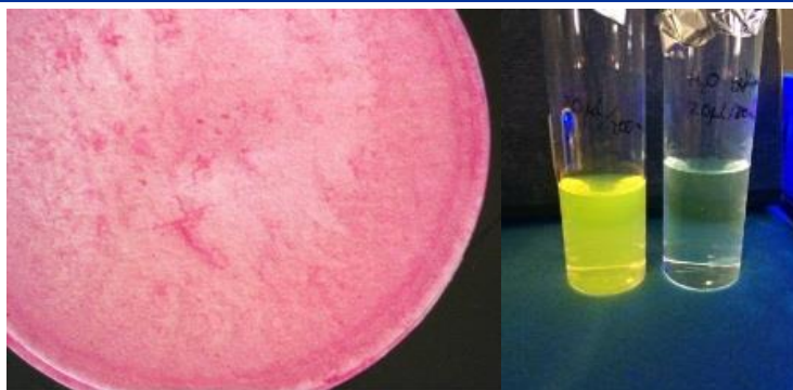
Figure 4. left-hand side: hybrid MMM after filtration, right-hand-side: fluorescence of the original solution and the filtrate under UV light illumination
