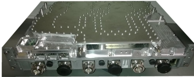
Figure 7. Nokia's liquid-cooled base station.
