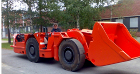
Figure 124. A 14-ton serial hybrid mining loader.
