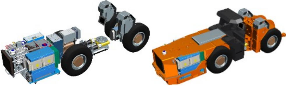
Figure 126. CAD drawing of the loader without and with body parts.
