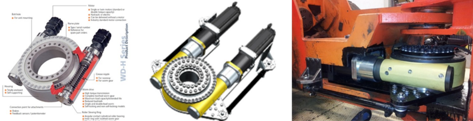
Figure 13. Electromechanical pivot steering with two servomotors and worm screw having some self-locking capacity. The behaviour in case of collision is one future question.
