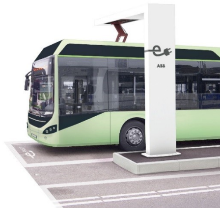
Figure 59. An electric bus with fast opportunity charging interface.
