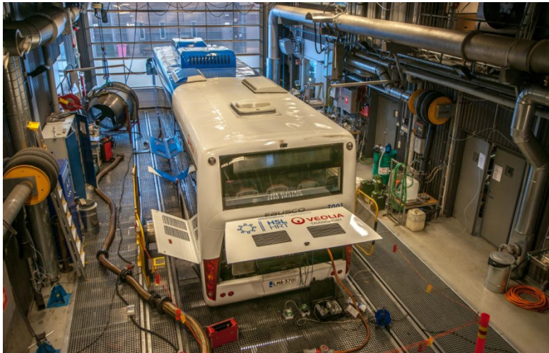
Figure 39. Heavy-duty vehicle test facility at VTT enables simulation of driving in a controlled laboratory.
