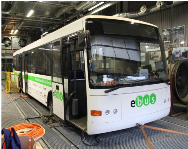
Figure 7. VTT's e-bus prototype and R&D platform being tested with VTT's heavy-duty vehicle dynamometer.
