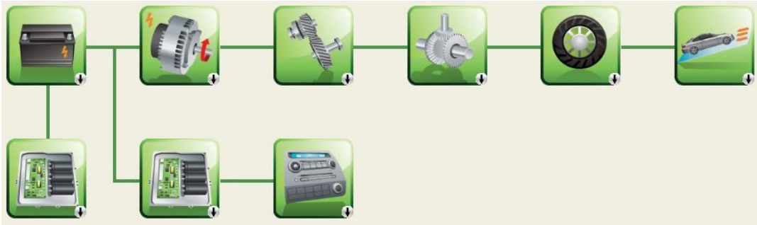
Figure 47. Powertrain layout. First row: Battery, Electric motor, Reduction gear, Differential gear, Wheels, Chassis. Second row: Charging device, Power converter, Auxiliary devices.
