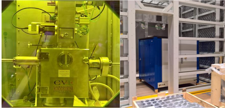
Figure 11. Since the electron beam welding takes place in a relatively small chamber (left), the large blue box containing the power supply and vacuum system was located in the rear of the cell in the new facilities (right), with only the e-beam column and vacuum chamber located inside the containment.
