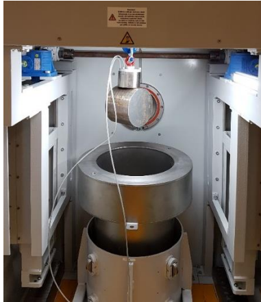
Figure 4. Testing manoeuvrability of a 40 kg dummy trepan as part of the evaluation if full trepans can be used for the investigations. The trials were successful.
