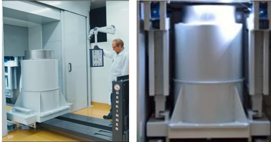
Figure 6. Site acceptance testing of the cask docking port of Cell 3.1 was carried out with a mock-up of VTT's existing vertically-oriented transport cask, and demonstrated good functionality of the system.
