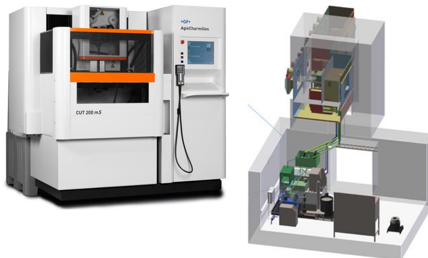
Figure 9. The EDM device (left) was special-ordered from the manufacturer such that the control panel could be separated from the cutting head and pool. At VTT the cutting unit is installed in Cell 1.1, and a special water circuit is deployed in the basement to enable separation of the radioactive cutting debris from the process water (right).
