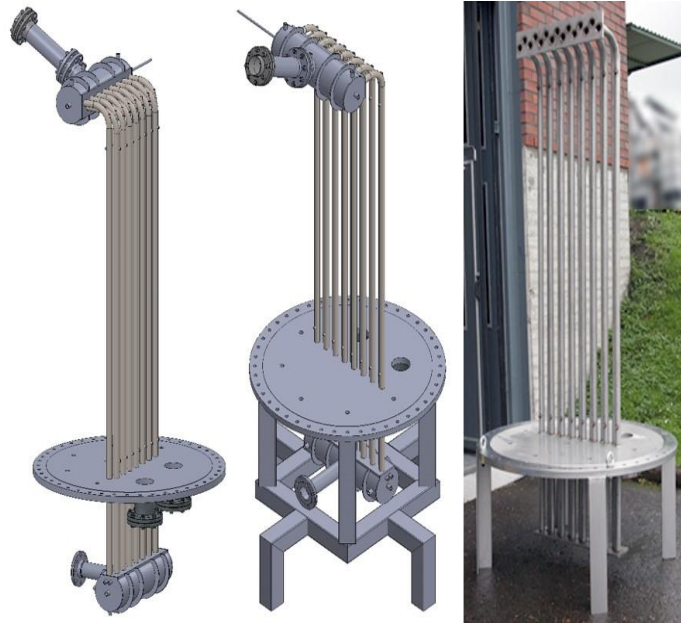
Figure 8. Heat exchanger of the PASI test loop.
