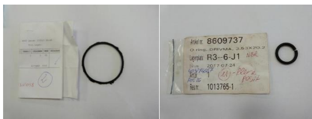
Figure 5. Two damaged O-rings from Ringhals to the left no EPDM and to the right no 11 NBR.
