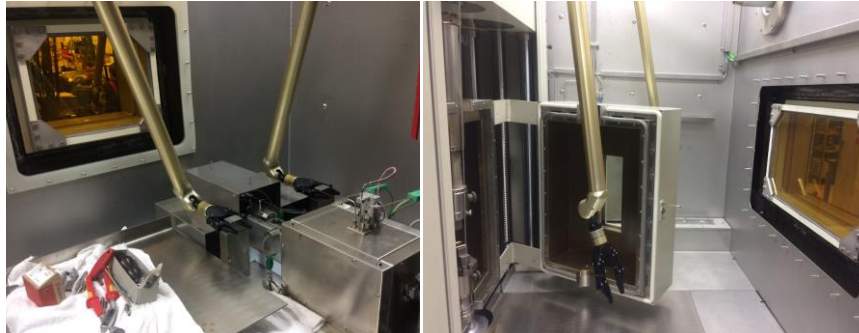
Figure 13. A Zwick HIT50 impact testing device (left) and Zwick Z250SW electro-mechanical tensile testing device (right) were fully integrated into Cell 1.4, including safety interlocks to prevent the impact hammer from accidentally hitting a stray manipulator (left).
