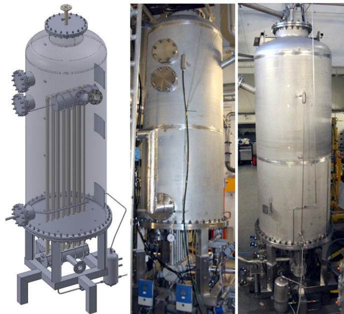
Figure 9. A pressure vessel of the PASI test loop simulating containment conditions.
