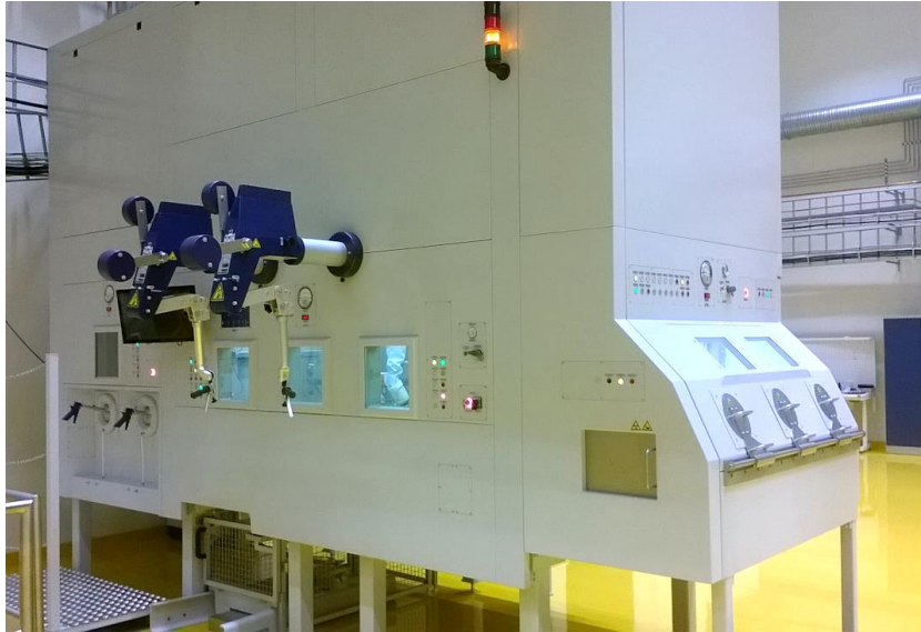
Figure 14. Module 2 is mainly for microscopy, and is comprised of three main compartments: LOM on left, specimen prep cell in middle, glove box on right end.
