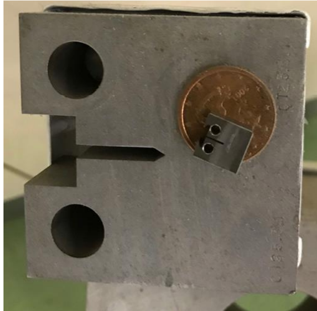
Figure 2. Newest innovation in surveillance specimen test techniques, miniature C(T) specimens. Four miniature C(T) specimens can be extracted from one Charpy-V specimen half.
