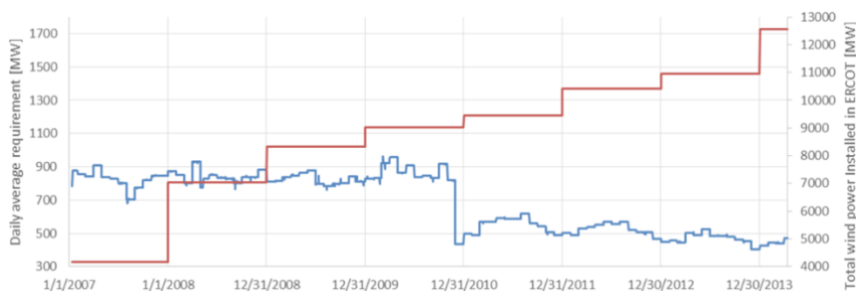
Figure 43. Up-regulation reserve requirement in ERCOT (blue) and total wind power capacity in ERCOT (red). (Source: The University of Texas at Austin energy institute, 2017)
