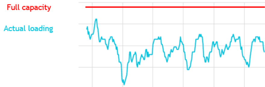
Figure 1. The difference between the nominal capacity and the actual loading of a heat exchanger.
