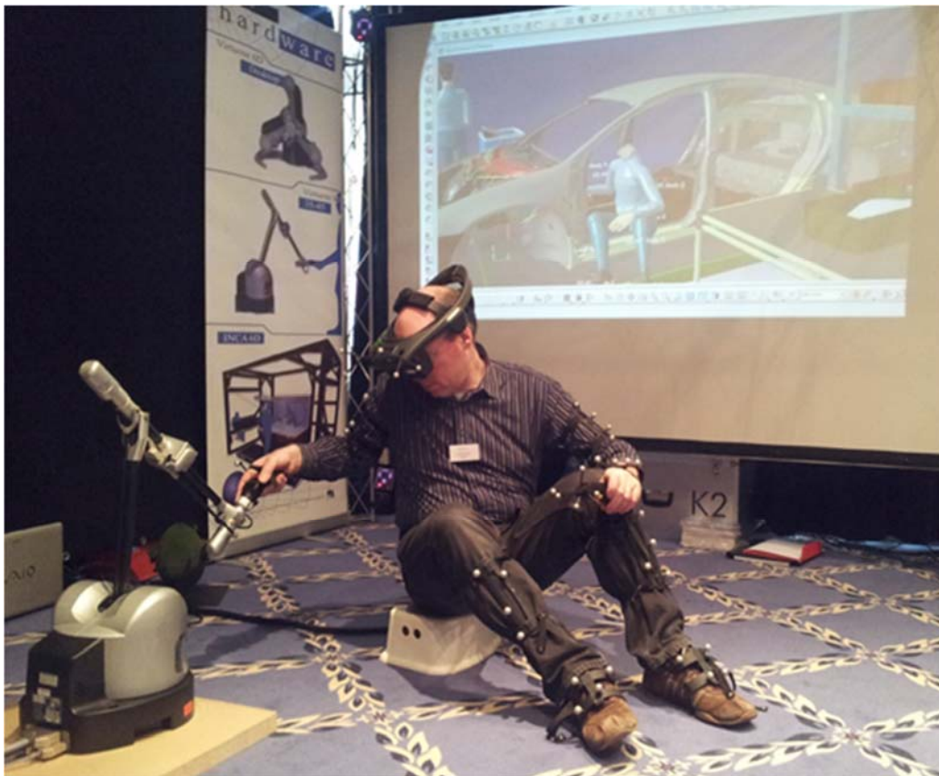
Figure 1. Combination of optical motion capture and force-feedback.
