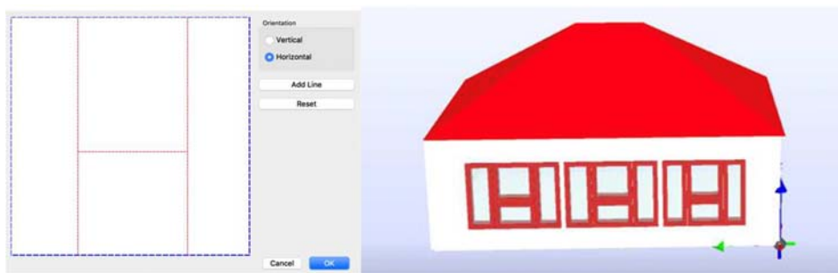
Figure 53. Detail editing of an opening and resulting opening
