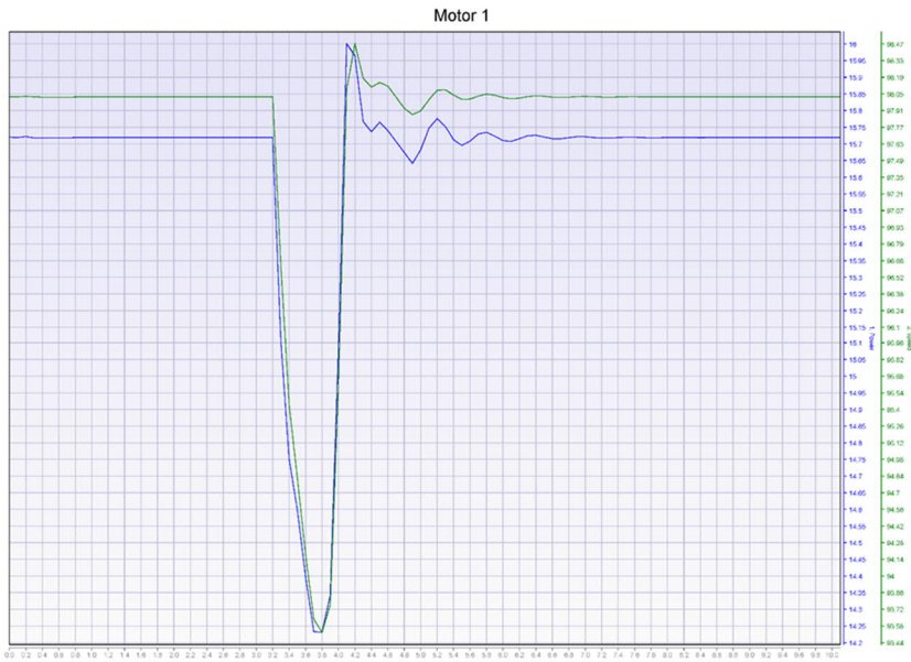
Figure 6. The mechanical power (kW) and angular speed (%) of the basic pump, modelled in Apros and coupled to asynchronous motor, modelled in Simulink.
