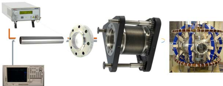
Figure 9.1. Measurement setup for testing the sensor at the North tokamak, DTU, Copenhagen.
