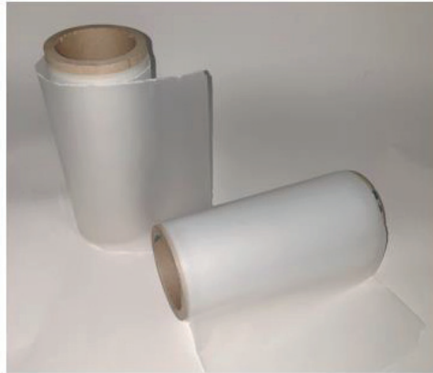
Figure 6.8 CNF film made of re-dispersed CNF
