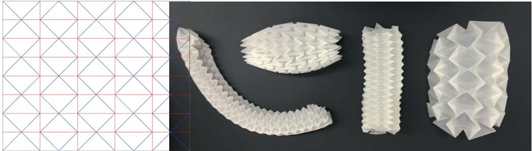
Figure P4. The Waterbomb base pattern and test pieces with different variations of the pattern.
