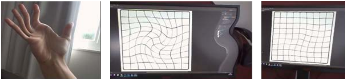
Figure 37. Sample system outputs as observed from the prototype. From left to right: the applied deformation, the input Amsler grid, the corrected Amsler grid.
