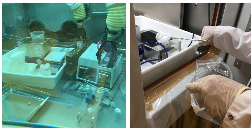
Figure 2. Cutting and grinding procedures when preparing microscopy specimens in the hot cells is a significant source of contamination and associated waste when cleaning up afterwards.
