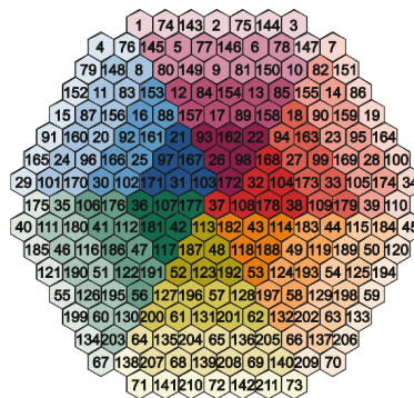
Figure 1. The mapping between the TRACE and PARCS models. TRACE nodes are mapped with different colors and the numbering corresponds to assembly numbering in PARCS.
