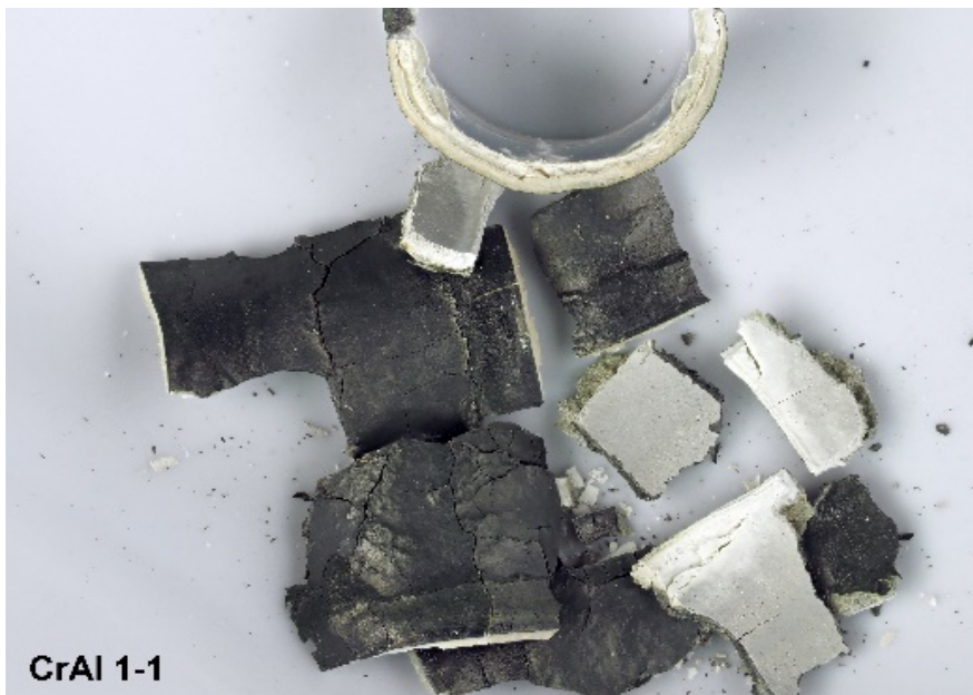
Figure 9. CrAl coated Zr-tube exposed at 1200 °C up to 30 min in flowing steam.
