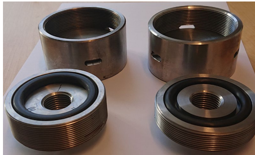
Figure 2. O-ring test rigs. Left: old test rig from COMRADE. Right: new test rig redesigned for SAMPO.
