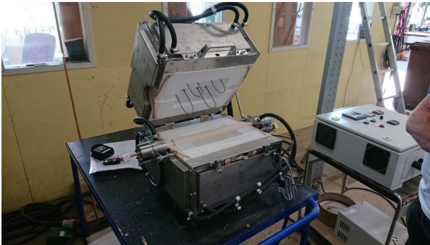
Figure 10. Furnace opened prior to the acceptance tests. The MoSi_2 resistive heating elements are attached to the furnace top cover. The sample tube lies on the bottom part of the furnace.
