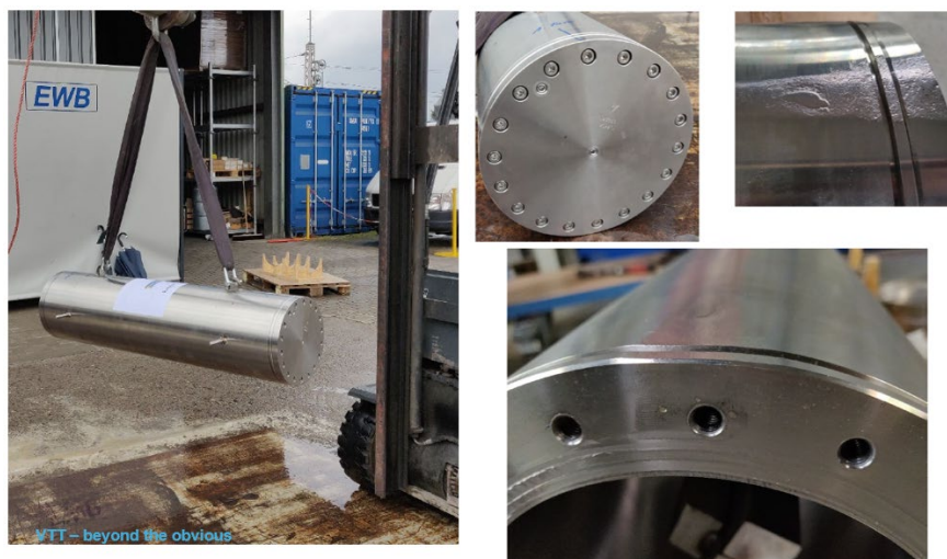
Figure 10. Certification of Daher GmbH's quality management plan for the A-Type road transport cask for irradiated materials involved conducting drop tests of 1:3 model of the cask during Q3/2020.
