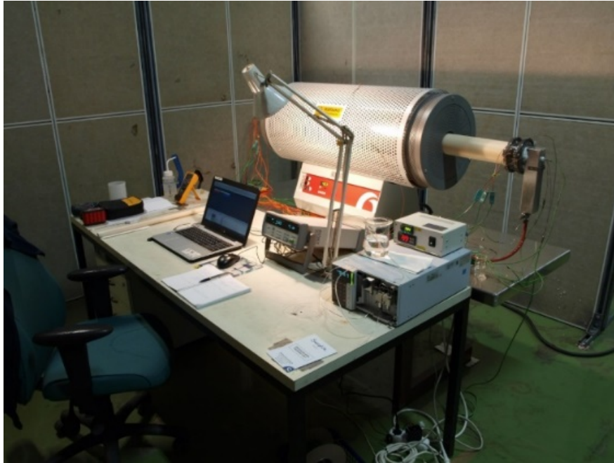
Figure 8. High temperature steam furnace system in VTT's Research Hall.
