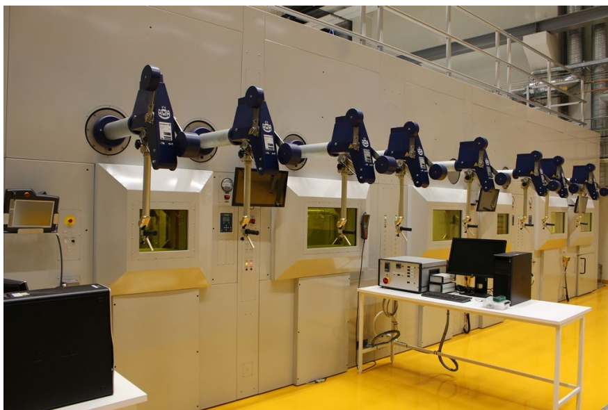
Figure 1. The new hot cells of the VTT Centre for Nuclear Safety were installed in 2017 during the SAFIR2018 program.
