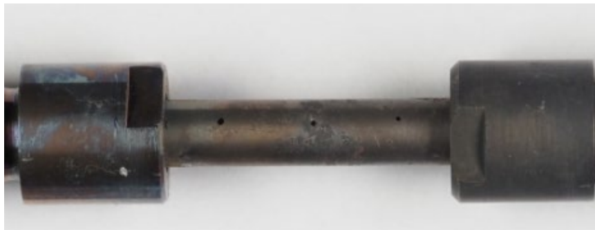
Figure 5. The creep specimen with length measurement in a) red dots indicating the diameter measurement locations in b) and black dots indicating the diameter measurement locations in c).
