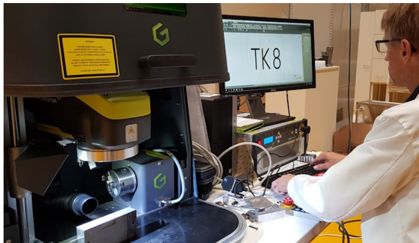
Figure 7. A laser engraving system was procured which enables precise, clean, durable marking of specimens with minimal damage.
