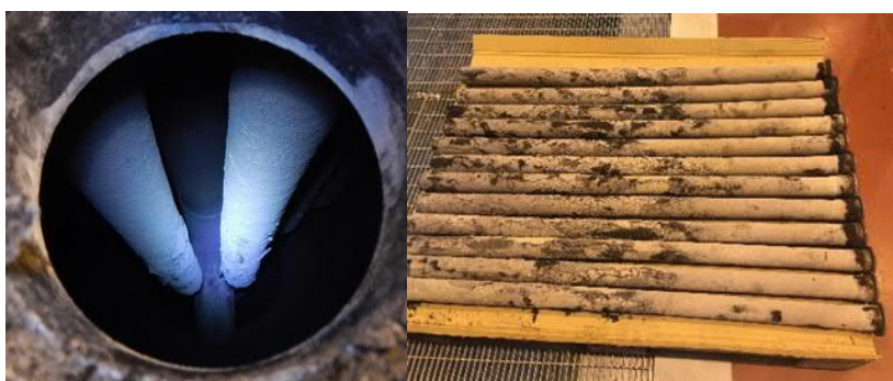
Figure 14. Photographs of the used filter elements after the last test run SXB 20/24.
