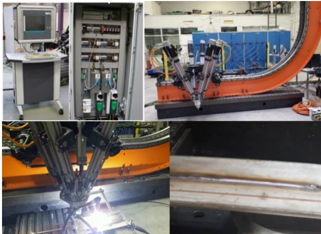
Figure 7.1. Mobile robotic machine for the assembly and maintenance of CFETR.
