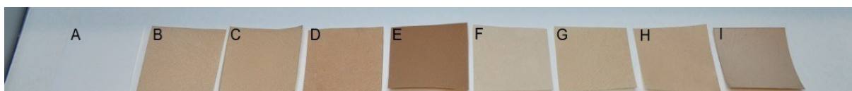
Figure 69. Photograph of LNPs-coated samples. A) pure Whatman 1 filter paper; (B-E) LNPs-coated samples prepared by immersion of filter paper into LNPs dispersions and (F-I) LNPs-coated samples prepared by spraying of filter paper with LNPs dispersions of 0.3 wt.-%, 0.5 wt.-%, 0.7 wt.-% and 2.6 wt.-% respectively.
