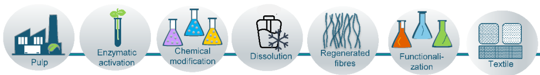
Fig.1. Process for producing functionalized Biocelcol textiles
