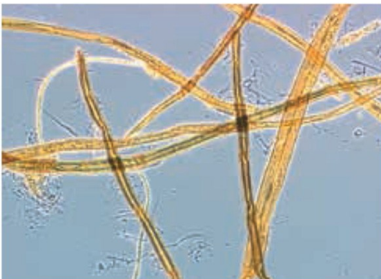
Figure 41. Refined fibres (left) and fibres with thin fibrils (crill) (right)
