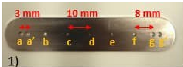
Figure 32. Locations of distribution plate holes
