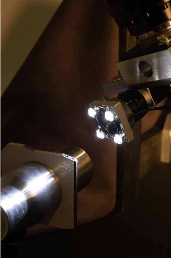
Figure 7.1: 3DNode camera system calculates the pose of an object
