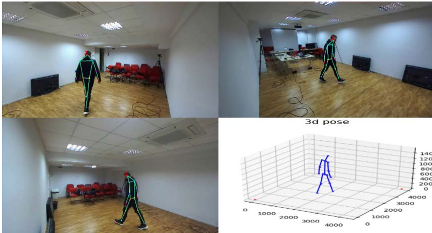
Figure 22. Projection of 3D poses and 3D visualization
