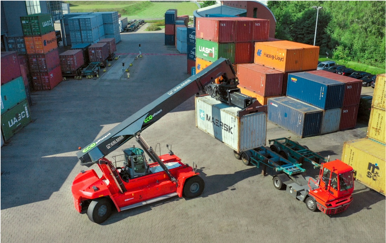
Figure 20. KALMAR reach stacker in operation
