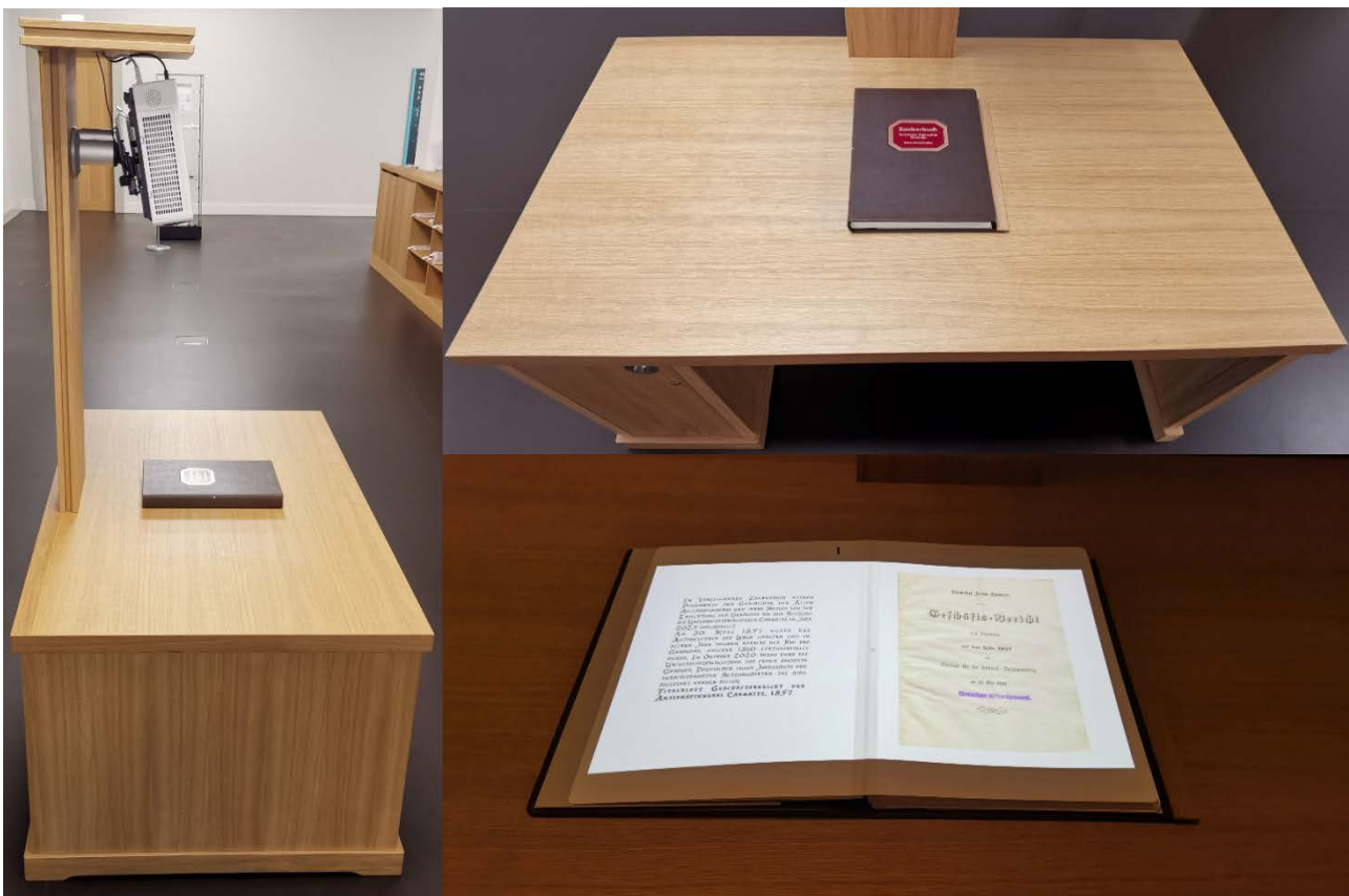
Figure 2. Left: Projective AR prototype "Zauberbuch", Top Right: The closed book from the users point of view, Bottom Right: Content of the first double page displayed on the book.
