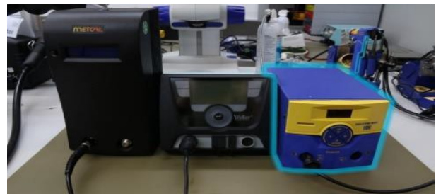
Figure 94. Easy Selection of Correct Solder Tool by Highlighting in Augmented Reality Glasses (Ansorge et. al., 2023)
