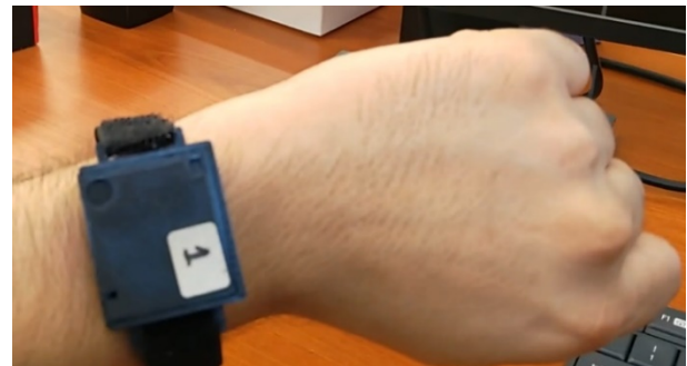
Figure 64. A special wearable is worn by the site's workers that tracks their location and their heartbeat at all times
