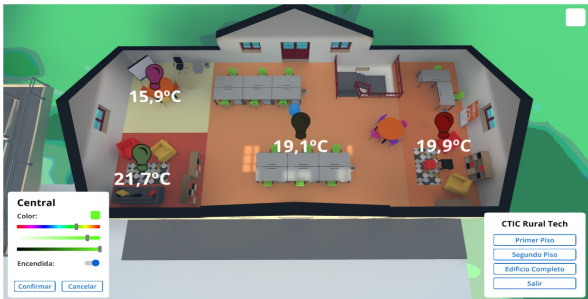
Figure 73 Office digital twin, home automation data monitoring and manipulation.
