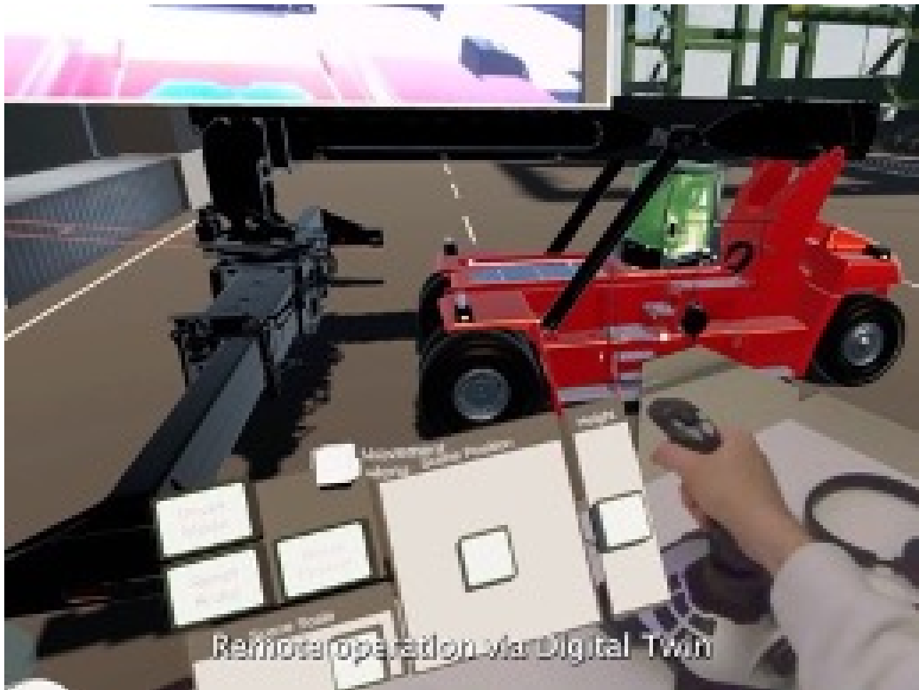
Figure 16. Mixed Reality based remote operation station which exploits Digital Twin (DT)
