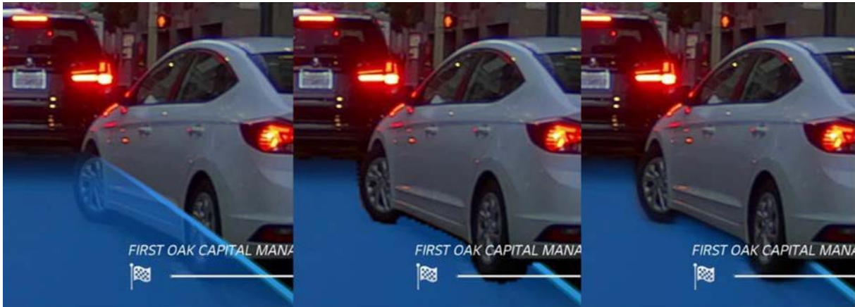
Figure 85. Removal of AR carpet overlap using semantic segmentation (left: overlapped, middle: overlap removed, right: overlap removed by smoothing and translucency effects)
