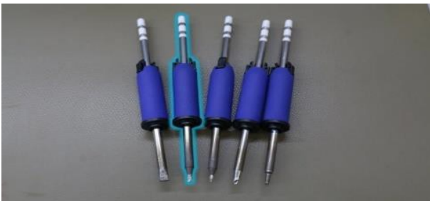
Figure 94. Easy Selection of Correct Solder Tool by Highlighting in Augmented Reality Glasses (Ansorge et. al., 2023)
