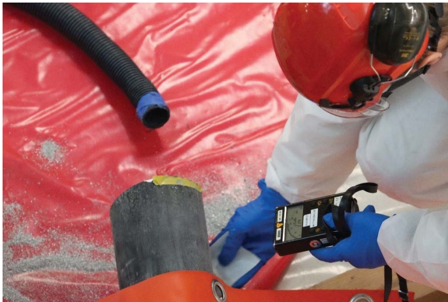
Figure 33. Activity measurements are done constantly to ensure right waste characterization and safe working methods.
