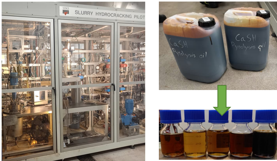
Figure 9. Left: Slurry hydrocracker pilot plant of RISE, Piteå. Right: pyrolysis oil feed and products of slurry hydrotreatment campaign.
