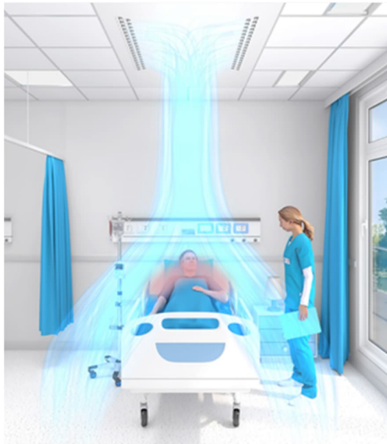
Figure 35 Protective airflow system concept, patient room
