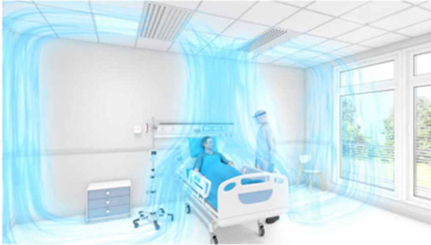
Figure 36 Protective airflow system concept, isolation room
