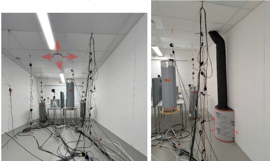
Figure 3. Basic ventilation cases: mixing ventilation (left) and displacement ventilation (right). Red arrows indicate the direction of air inlet.
