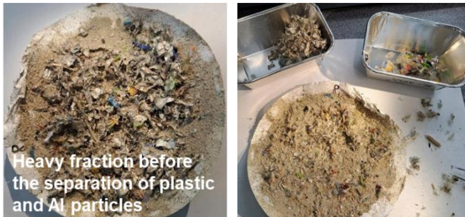
Figure 3. Example of manual determination of PE and Al content of the heavy fraction.
