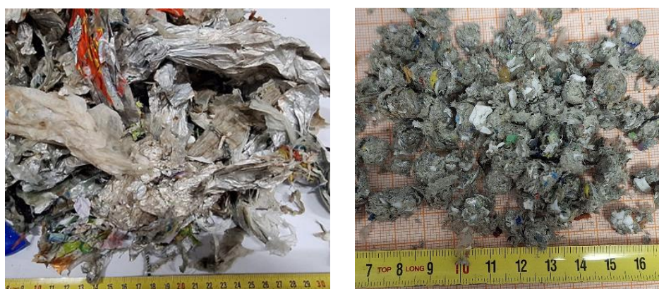
Figure 19. The original feedstock (left) and pelletized plastic reject (right).
