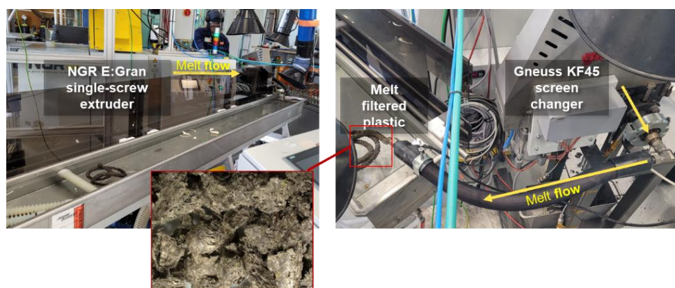
Figure 12. Melt filtration of light plastic fraction from WP1.
