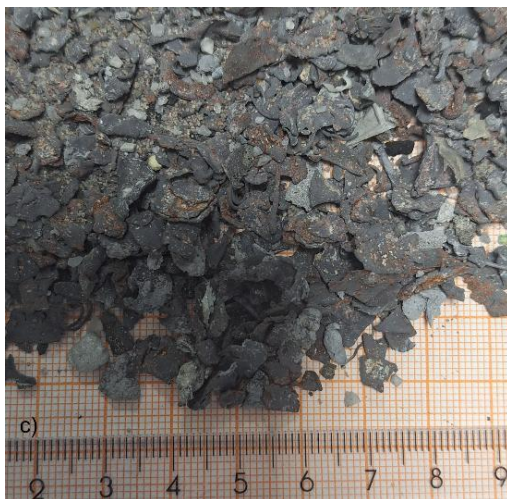
Figure H3. Particles collected from the gasifier plate distributor after
