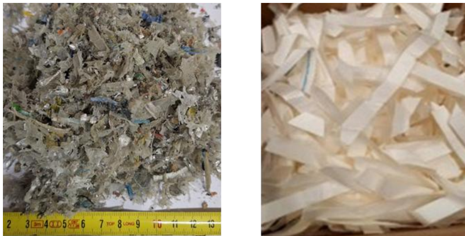
Figure 2. Plastic waste with aluminium and fiber residues (left) and cupboard with fiber material and PE (right).
