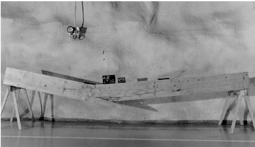
Failure behaviour of specimen (49 H) in series LT-A2-H5a-10.
