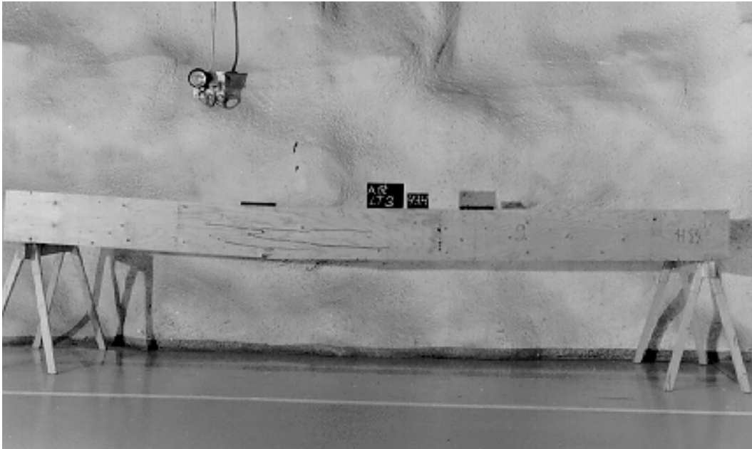
Failure behaviour of specimen (43 H) in series LT-A2-H5a-1.
