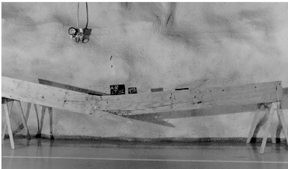
Figure 24. Failure behaviour of beam 49H in LT-A2-H5b series.
