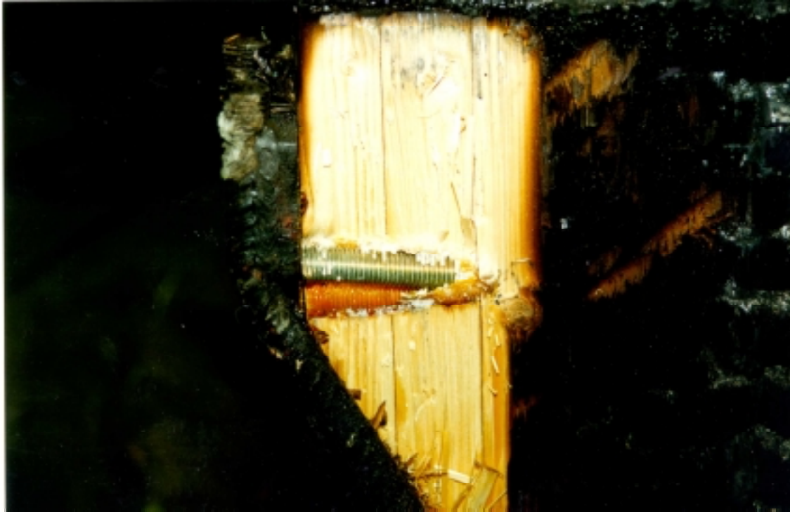
Figure 14. Failure of timber in beam 2 after the test.
