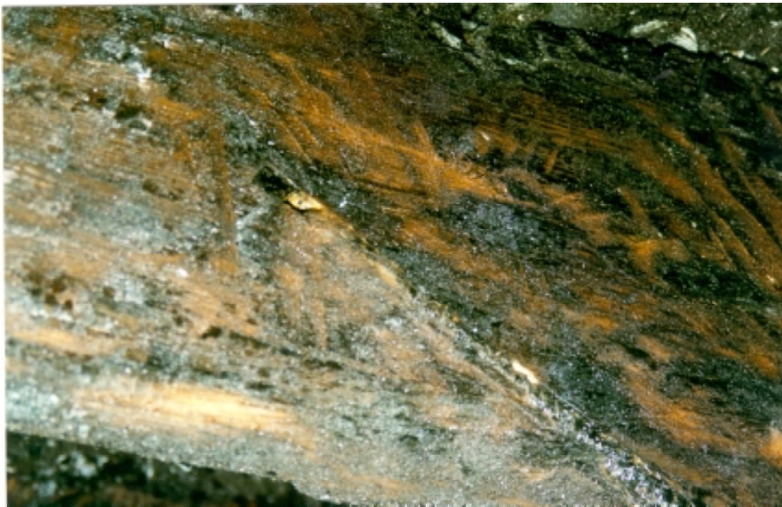
Figure 13. The slip of the steel rod in beam 2 after the test.
