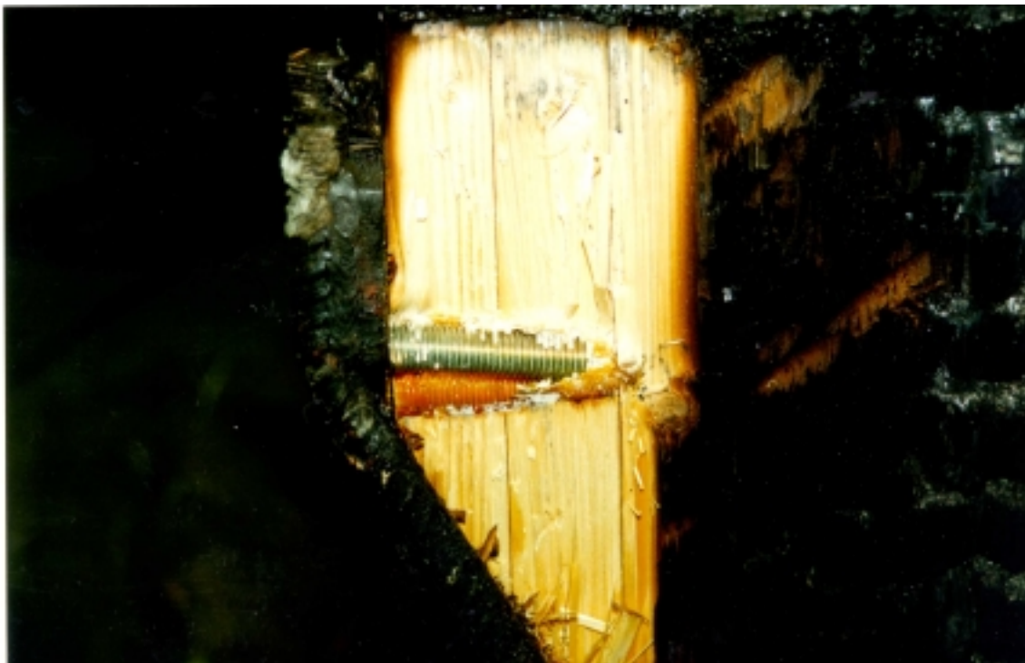
Figure 17. Failure of wood in Beam 2.
