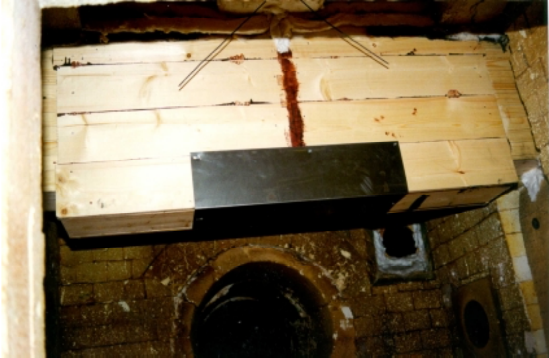
Figure 11. Furnace test set-up.
