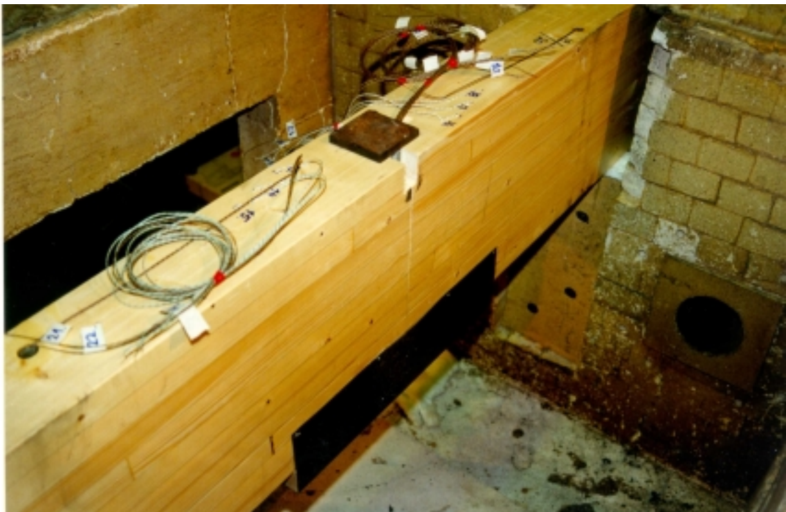
Figure 3. Test arrangements in the furnace.
