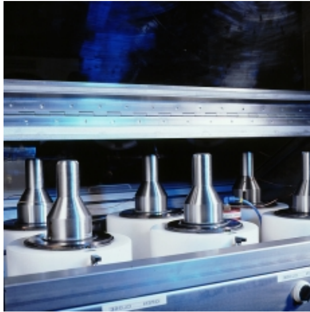
Fig. 1. A laboratory- scale high pressure equipment suitable for kinetic studies as well as for product development.
