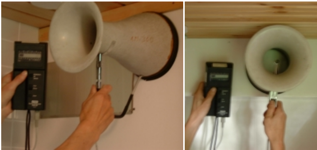
Figure 69. Measuring the exhaust flow rate.
