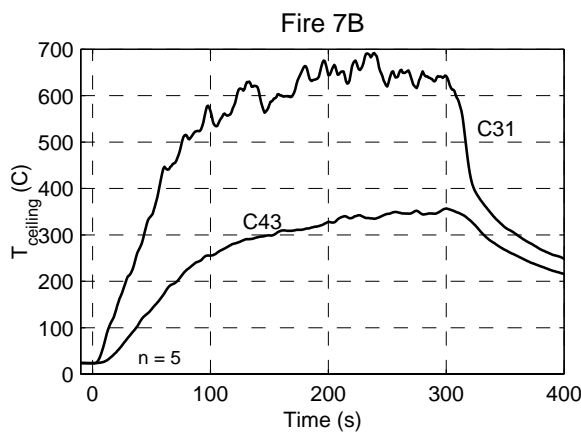
Figure 37e. Ceiling jet temperatures.
