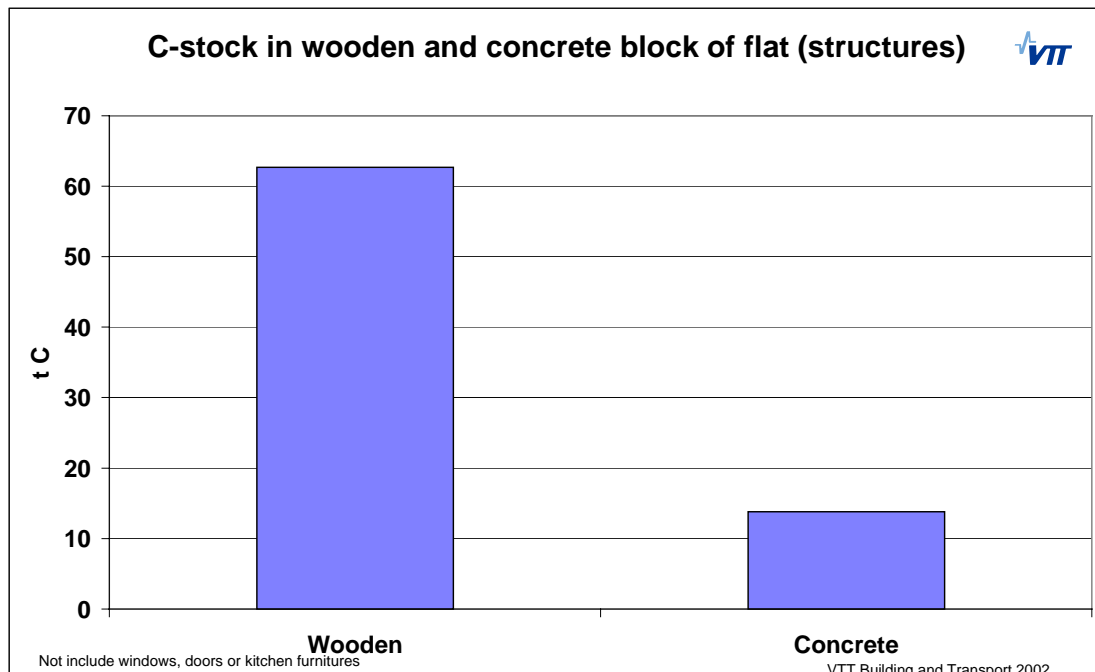
Figure 15. The C stock of HWP in the wooden block of flats in Viikki and the corresponding C stock of similar house built from concrete.
