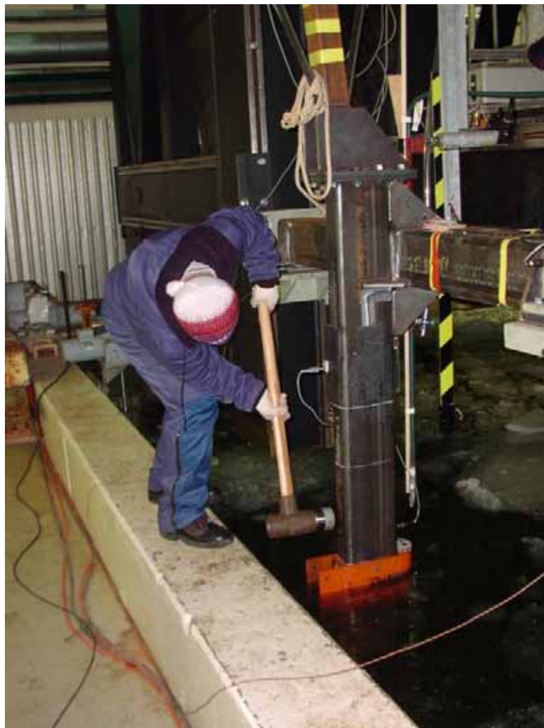
Figure 26. Hammer blow excitation in direction "a" by Bi Xiangjun.
