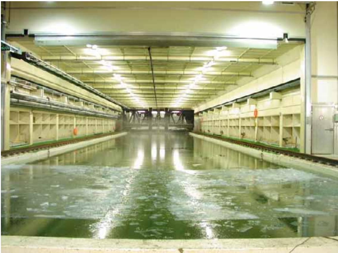
Figure 1. HSVA's 78 m long, 10 m wide and 2.5 m deep ice basin.
