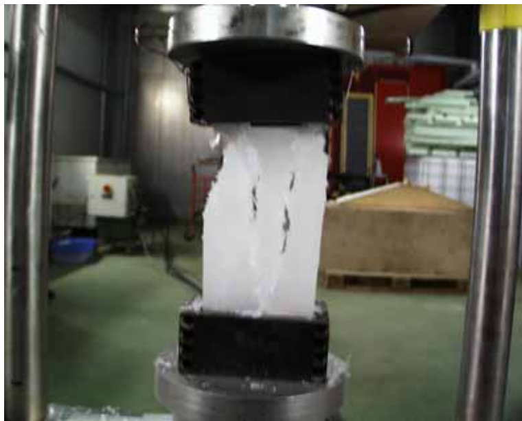
Figure 28. Uniaxial compressive test.
