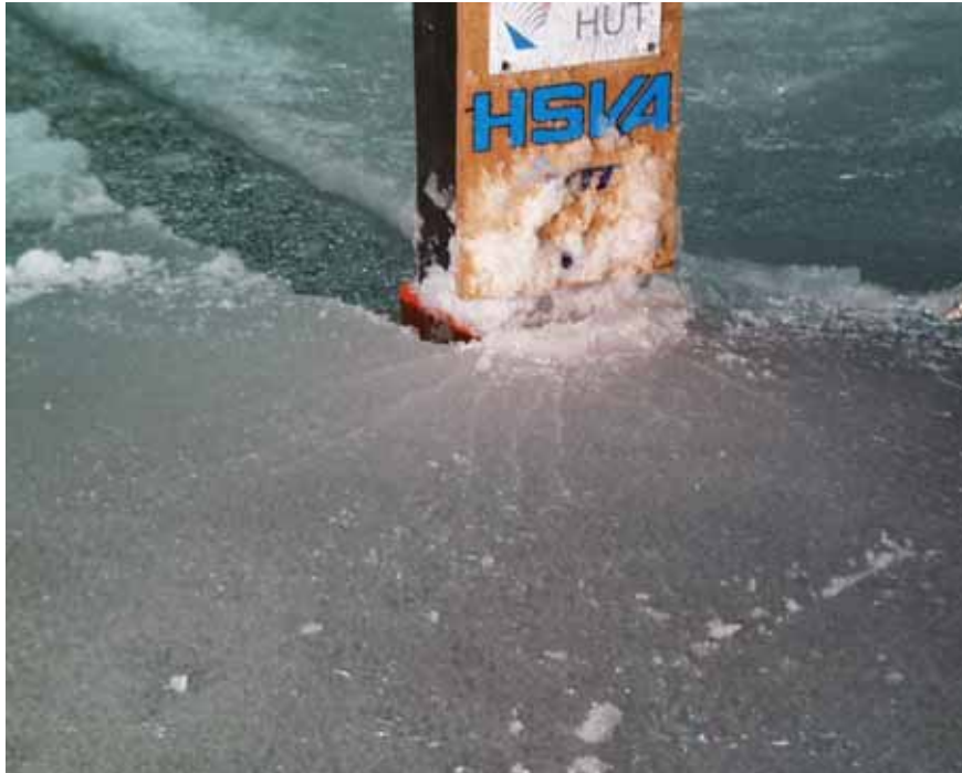
Figure 34. Ice failure in front of the inclined indenter.
