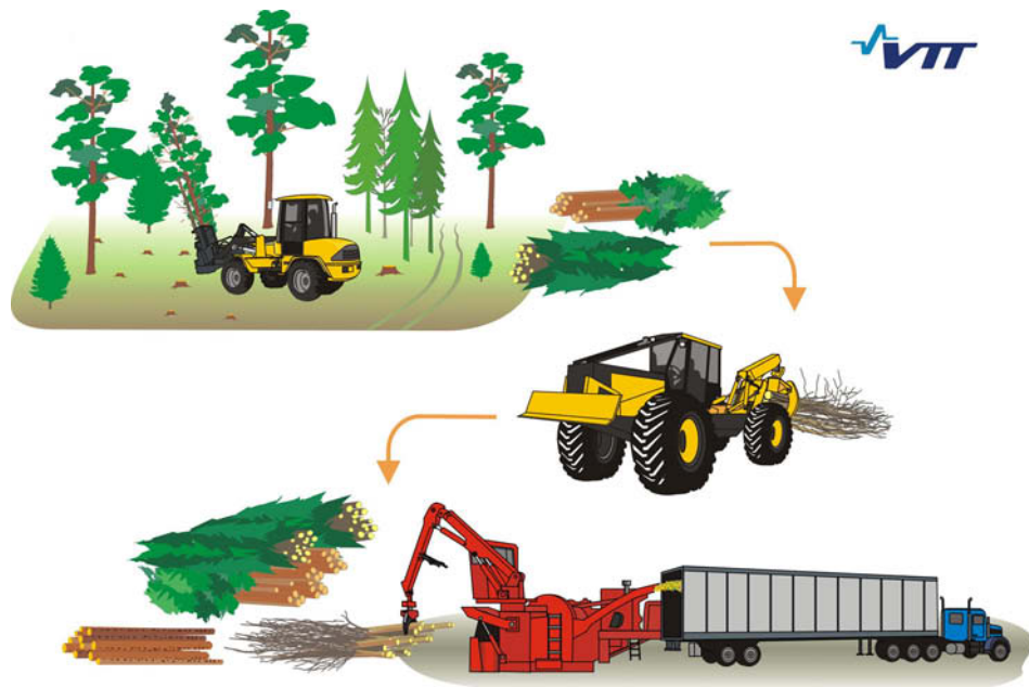
Figure 8. Principle of the whole tree – fuel chip harvesting chain (Arola & Miyata 1981).
