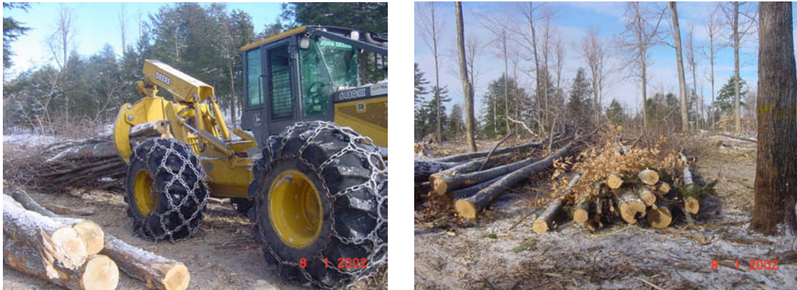
Figure 11. Grapple skidder (John Deere) and bunches at a landing in Vermont (photos by Arvo Leinonen).
