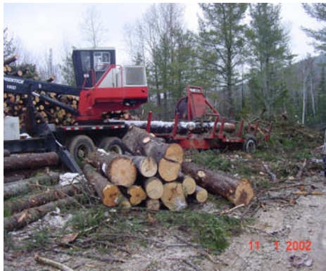
Figure 3. Some processing equipments of whole trees at road site or landing – slasher (photo by Arvo Leinonen) and Morbark 2755 Flail Chipharvestor (Morbark 2002).
