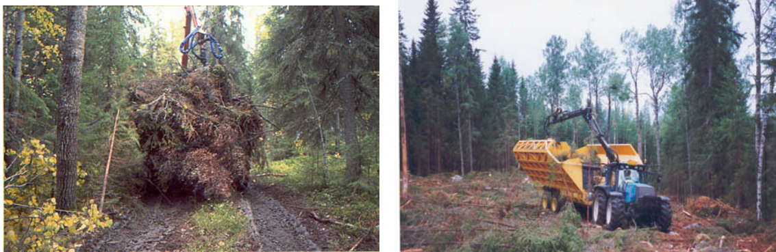
Figure 22. Haulage of forest residues with forwarder (left) and with Havu-Hukka-trailer (right).
