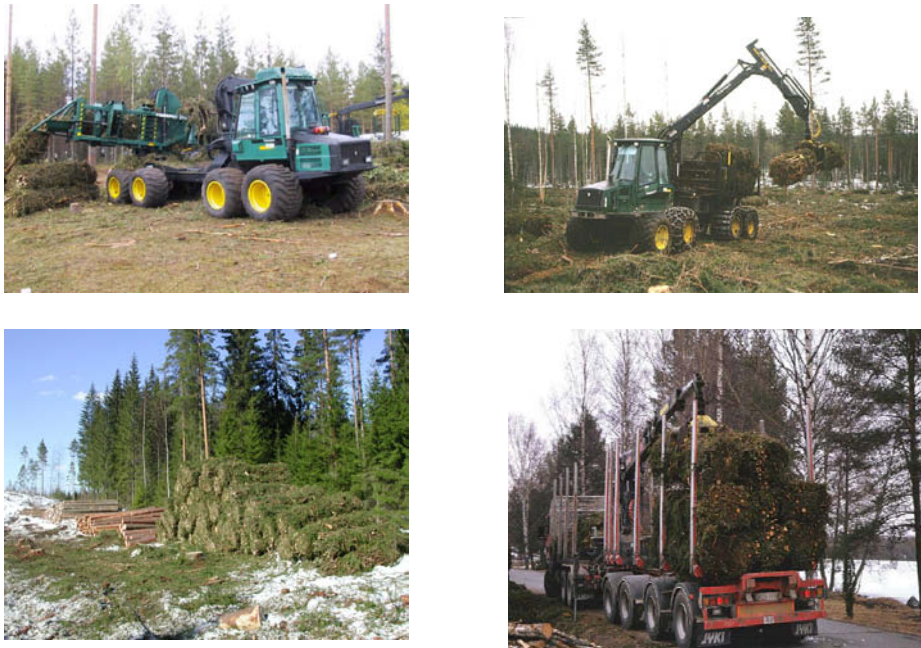
Figure 29. The bundling technology chain – bundling (left above), terrain hauling (right above), storage (left below) and road transport (right below).
