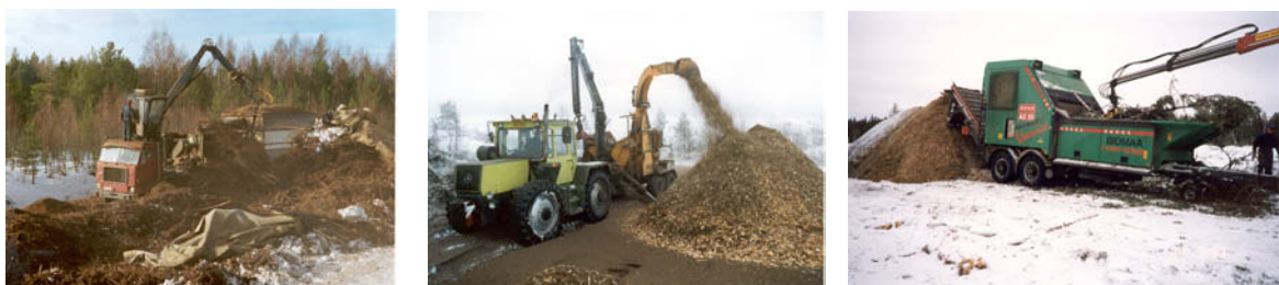
Figure 24. A mobile chipper on a truck chassis (left), a mobile tractor chipper (in the middle) and a crusher (right) (photos by VTT Processes).
