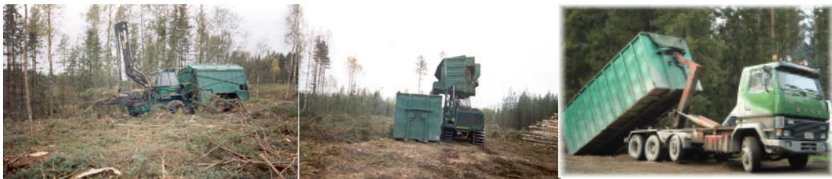
Figure 27. Harvesting chain of forest residues based on the terrain chipper – harvester (left), loading of chips into the exchangeable container (in the middle) and loading of the container for truck transport to power plant (right) (photos by Arvo Leinonen and Biowatti Oy).
