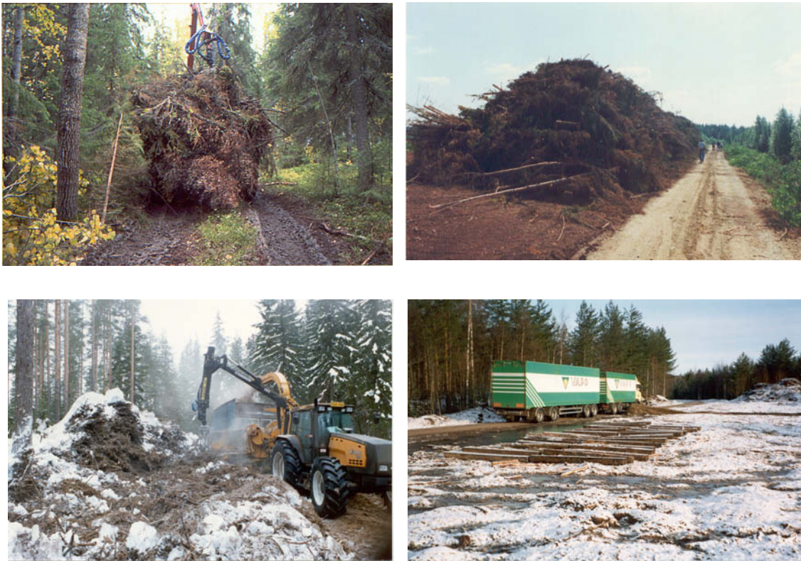
Figure 21. The forest residues harvesting chain based on chipping at the roadside landing – terrain haulage (left above), storage (right above), chipping into truck trailer (left below) and truck trailer road transport (right below) (photographs by VTT Energy).
