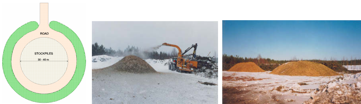
Figure 26. A schematic picture of a circular terminal (left), chipping at circular terminal (in the middle) and storage of forest residue chips at terminal (right) (Leinonen et al. 2000).
