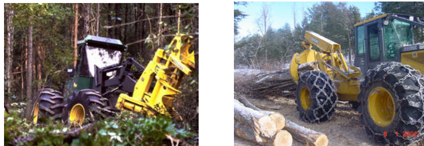
Figure 2. Whole-tree harvesting chain – drive-to-tree feller buncher Timberjack 740 feller buncher (left) (photo by Timberjack) and grapple skidder (right) (photo by Arvo Leinonen).
