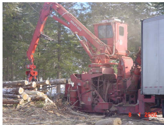
Figure 12. Tops and small tree pile for fuel (left) and Morbrak M 30 drum chipper chipping into the trailer (right) at a landing in Vermont (photos by Arvo Leinonen).
