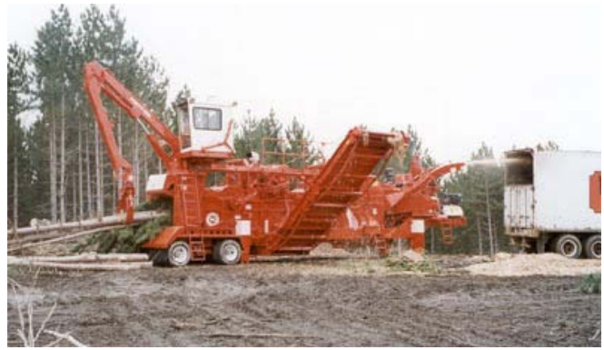
Figure 3. Some processing equipments of whole trees at road site or landing – slasher (photo by Arvo Leinonen) and Morbark 2755 Flail Chipharvestor (Morbark 2002).
