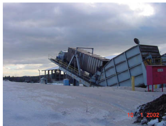
Figure 14. Chipper is blowing the chips into a truck trailer at a landing (left) and a truck is under unloading station at a power plant (right) (photos by Arvo Leinonen).
