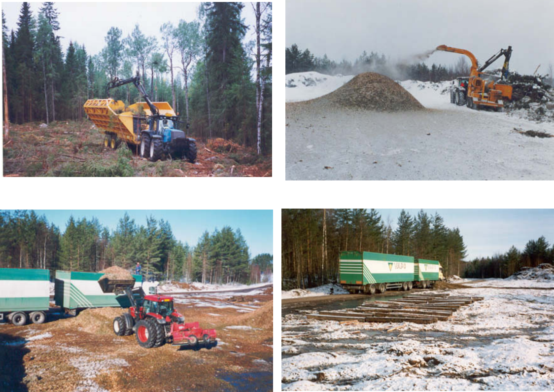
Figure 25. Forest residue harvesting chain based on chipping at the fuel terminal – terrain haulage with Havu-Hukka trailer (left above), storage and chipping (right above), truck loading (left below) and truck trailer road transport (right below) (photos by VTT Processes) (Leinonen et al. 2000).
