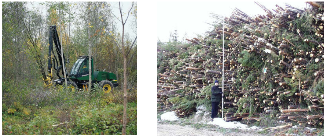
Figure 31. Thinning harvester (left) and small trees for wood fuel in a storage (right) (photos by Arto Timperi, Timberjack and Kari Hillebrand, VTT).
