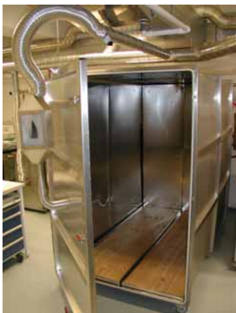
Figure 4. 5-m 3 stainless steel chamber for emission testing.
