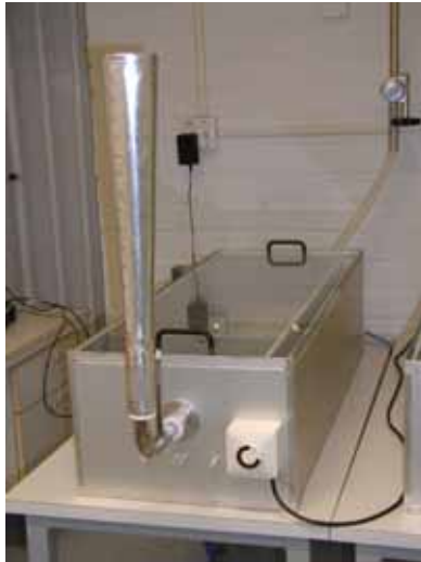
Figure 3. Example of a diffusor-equipped test chamber for sensory testing of building materials.
