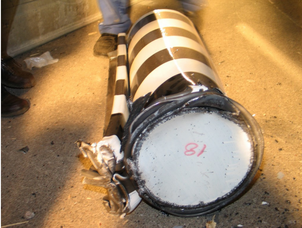
Figure 62. Deformed preliminary missile.
