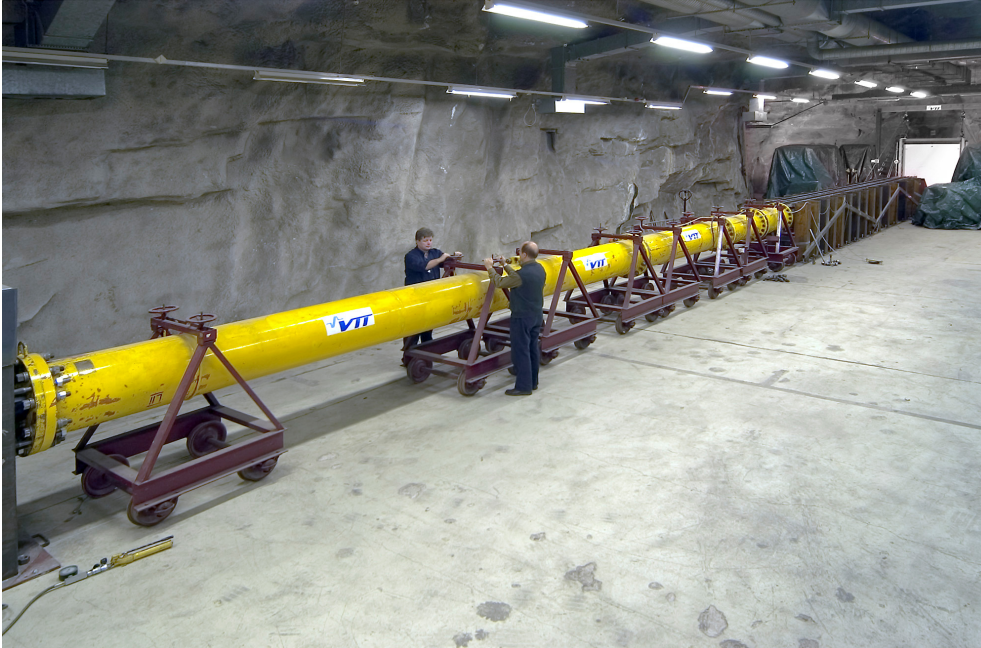
Figure 60. Apparatus for impact tests, installed in an underground space.
