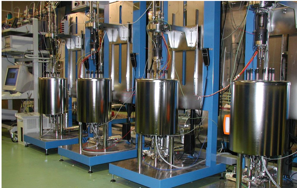
Figure 36. Four fatigue autoclaves in a hot water circulation loop.
