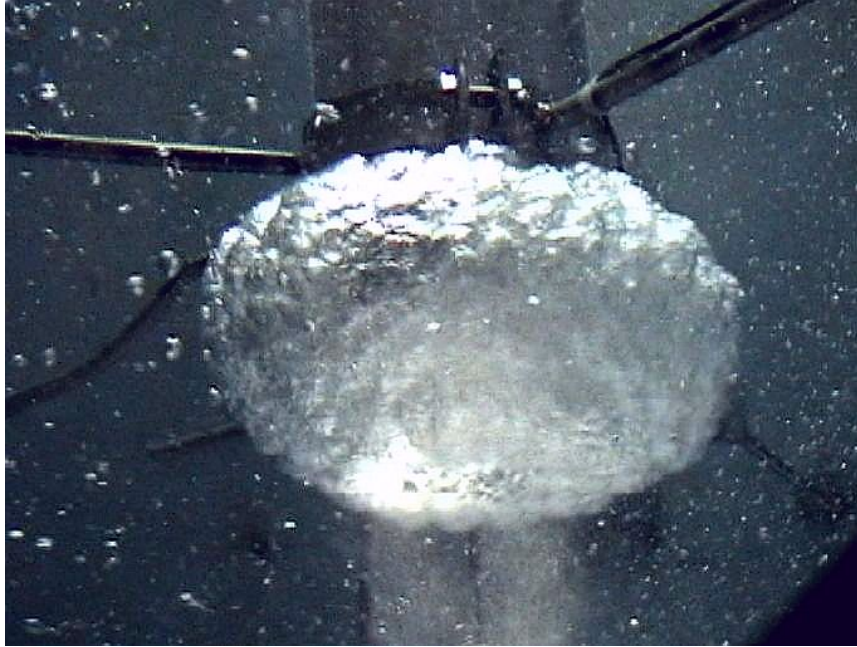
Figure 99. Steam bubble forming at the DN200 blowdown pipe outlet.
