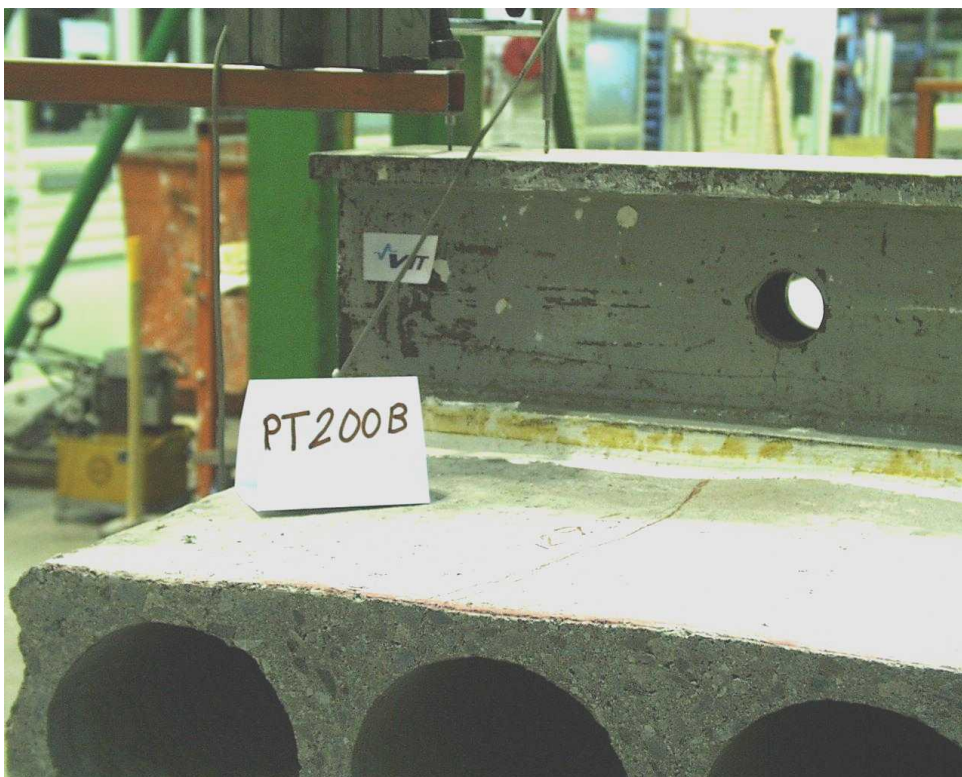
Fig. 18. PT200B. Cracking of cantilevered passive end.
