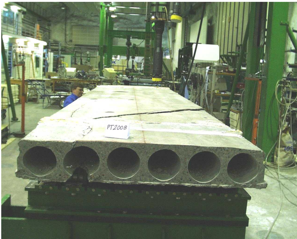
Fig. 22. PT200B. Cracking pattern after removal of loads and loading equipment.
