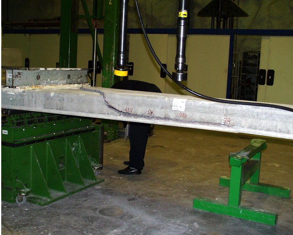
Fig. 15. PT200A. Cracking pattern after failure. The red figures refer to the applied actuator load.
