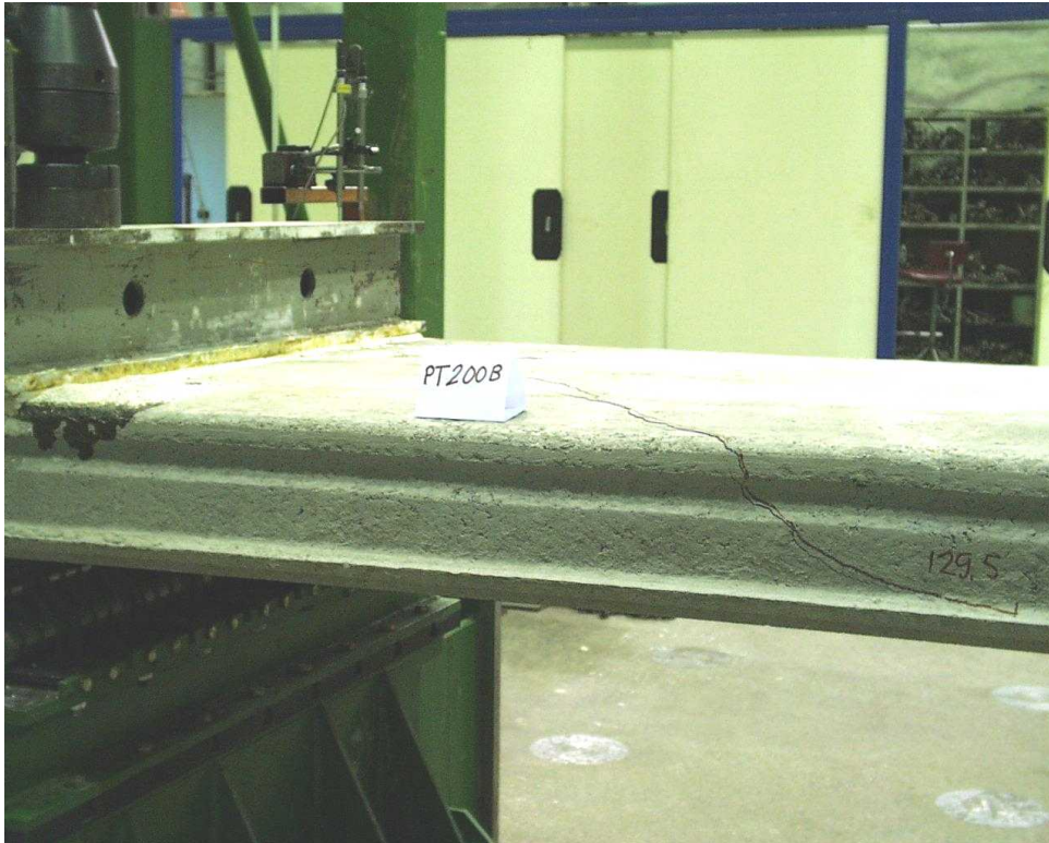
Fig. 17. PT200B. Cracking pattern at passive end.
