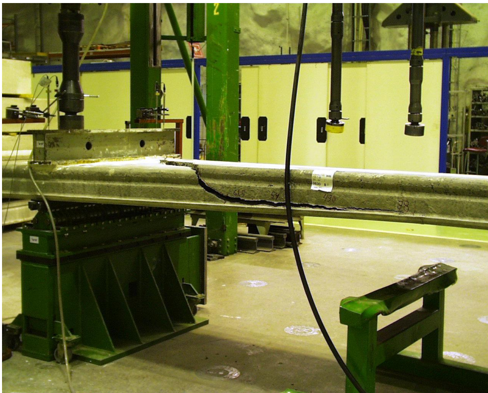
Fig. 10. PT200A. Side view after failure.
