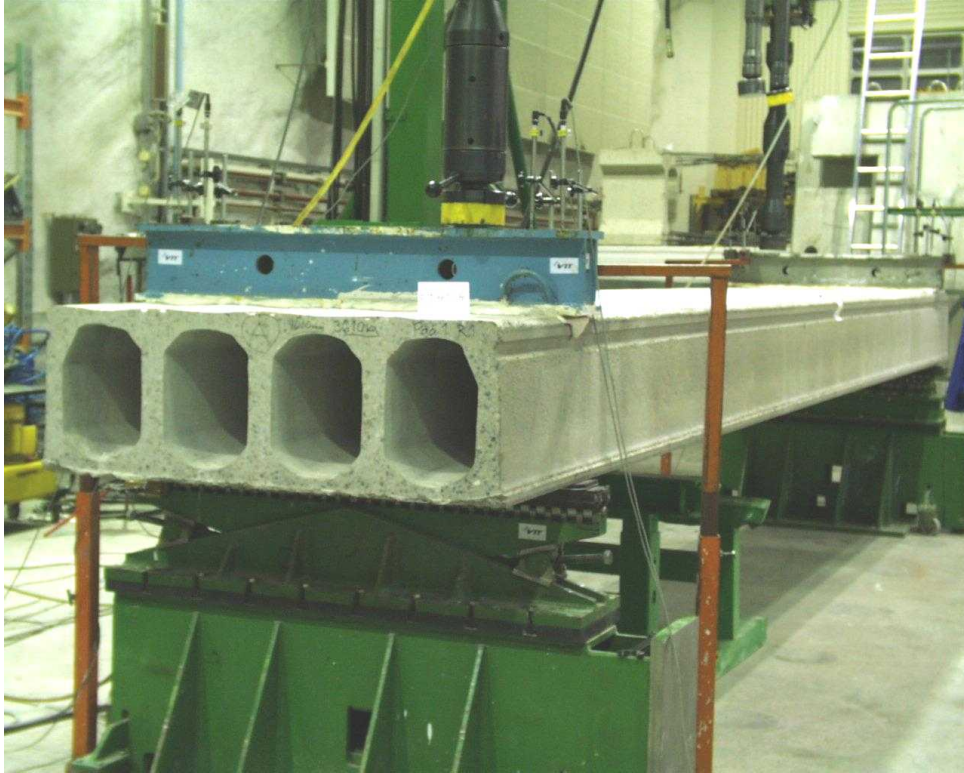
Fig. 25. PT400A. General view on the test layout.
