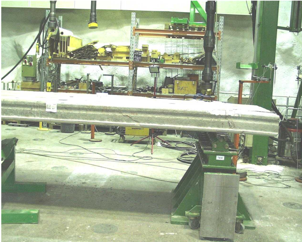
Fig. 23. PT200B. Cracking pattern after removal of loads and loading equipment.
