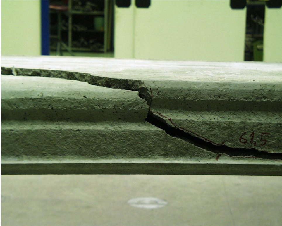
Fig. 9. PT200A. Detail of crack after failure.
