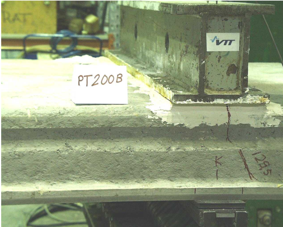
Fig. 19. PT200B. Cracking below the spreader beam at passive end.
