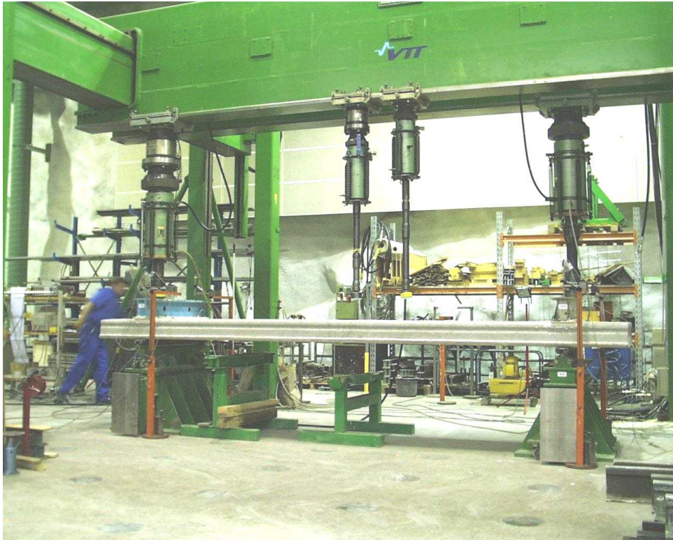
Fig. 5. PT200A. Side view on test arrangements. The two actuators in the middle were not used.
