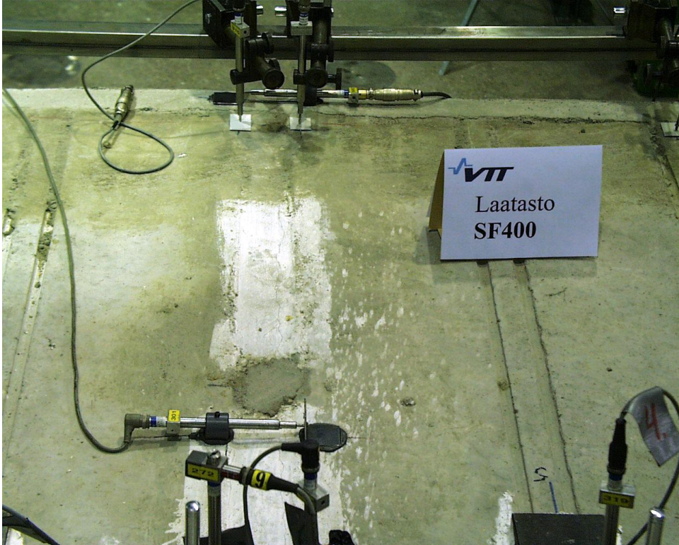
Fig. 7. Horizontal transducers for measuring crack opening.
