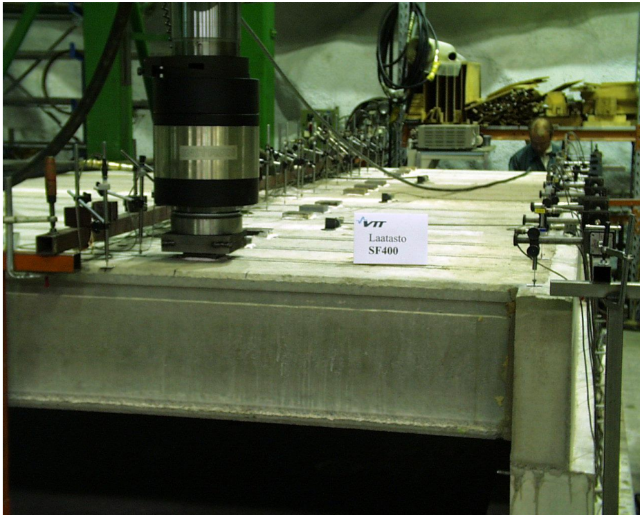
Fig. 8. Load at the edge of the floor.
