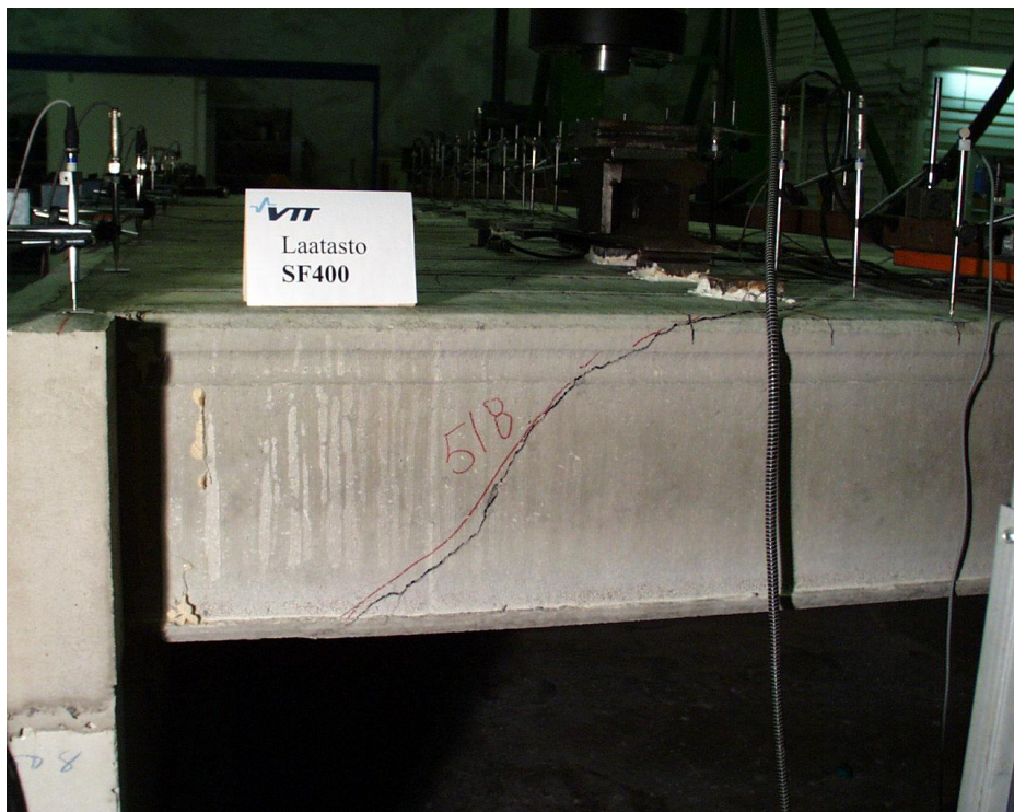
Fig. 30. PF400:15. Cracking after failure.
