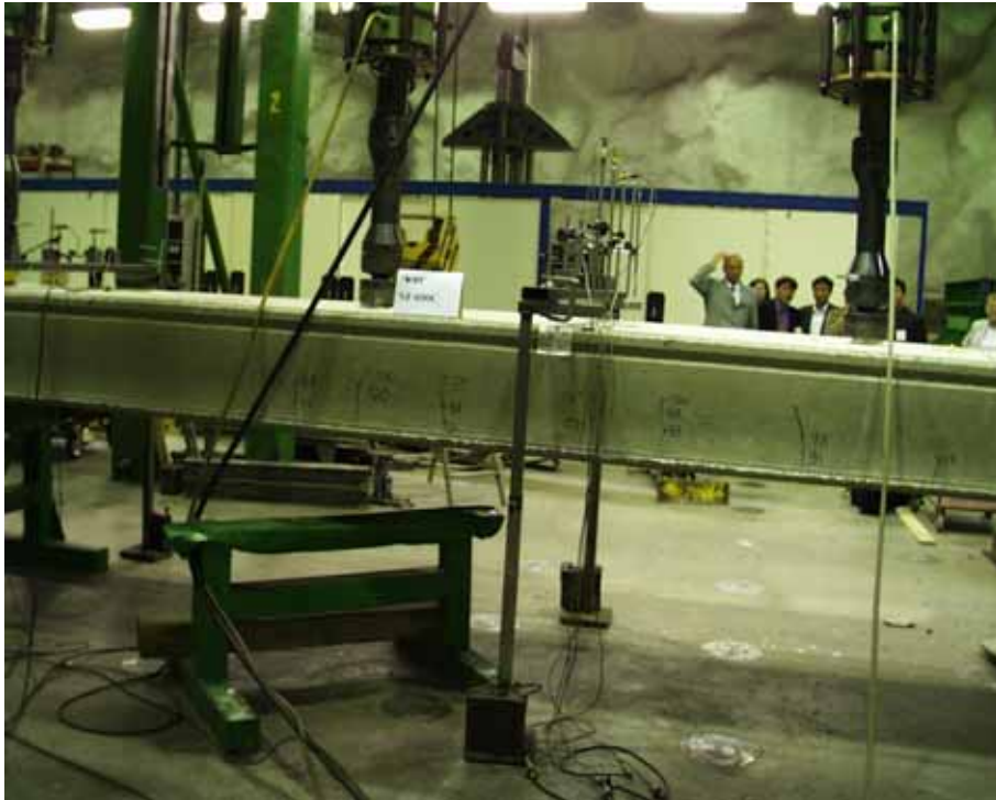
Fig. 35. SF400C. Flexural cracks in mid-span, Southern edge.
