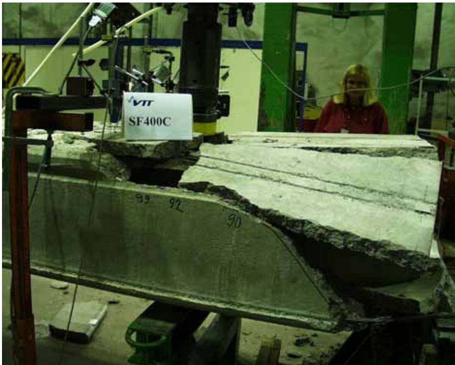
Fig. 30. SF400C. Southern edge after failure. Before loading there was an initial crack above the first hollow core in the front. It extended \approx 450 mm from slab end to the span.
