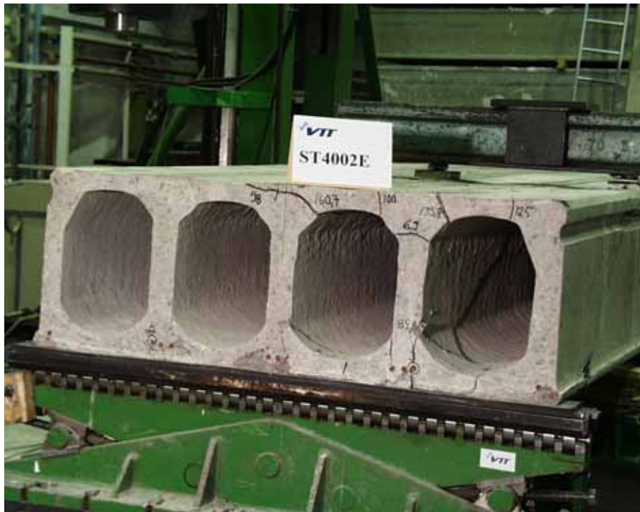
Fig. 24. ST4002E. Cracks in webs after failure.
