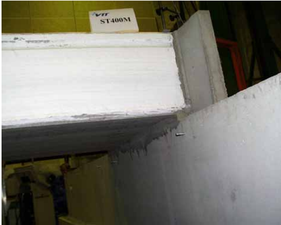
Fig. 37. ST400E1M. Well-compacted grout below the slab end.
