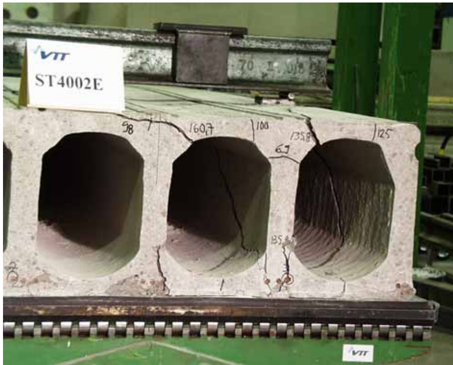
Fig. 23. ST4002E. Cracks in webs after failure.
