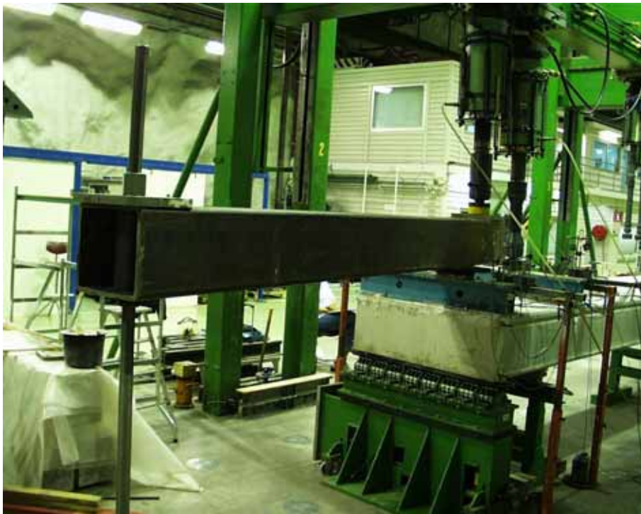
Fig. 46. ST400G. Auxiliary beam for creating eccentric load at sheared end.
