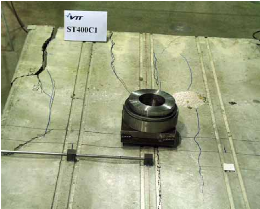
Fig. 5. ST400C1. Top surface after failure. Note the letter A on the upper left corner of the figure. Before loading there was an initial crack from the slab end to letter A.
