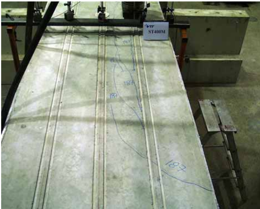
Fig. 40. ST400E1M. Cracks on the top after unloading.
