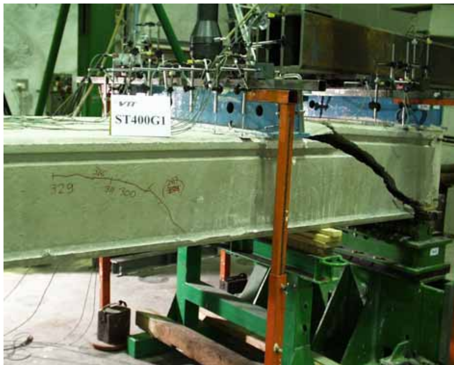
Fig. 52. ST400G1, North edge, cracks after failure.
