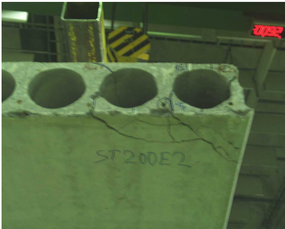
Fig. 24. ST200E2. Soffit after failure.
