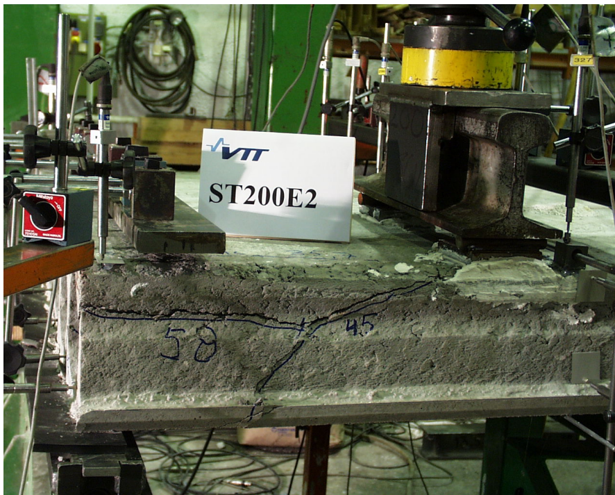
Fig. 22. ST200E2. Cracking pattern after failure. Northern edge.
