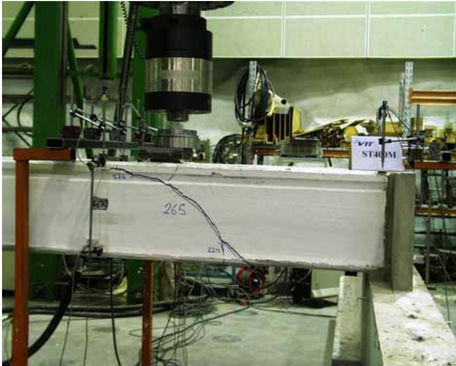
Fig. 39. ST400E1M. Shear crack after unloading.
