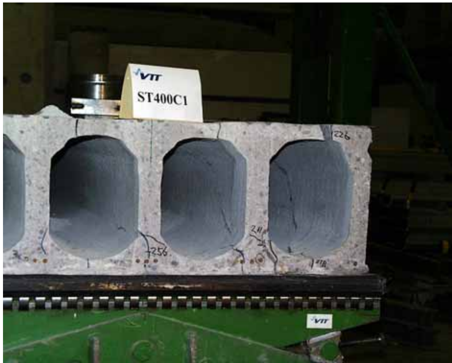
Fig. 4. ST400C1. Cracks in webs after failure.
