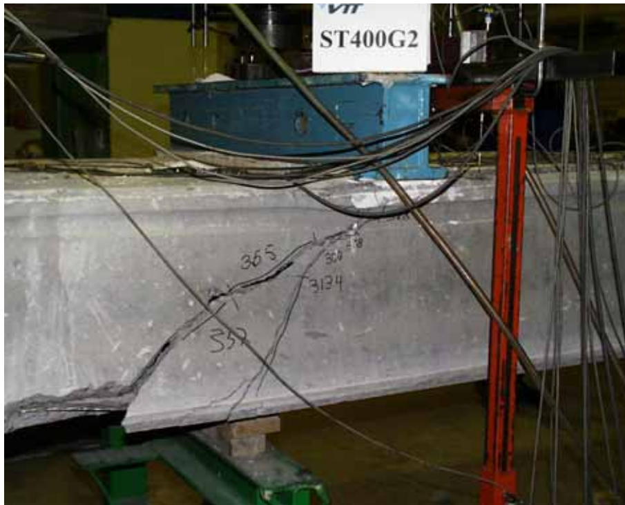
Fig. 61. ST400G2, South edge, detail of failure cracks.
