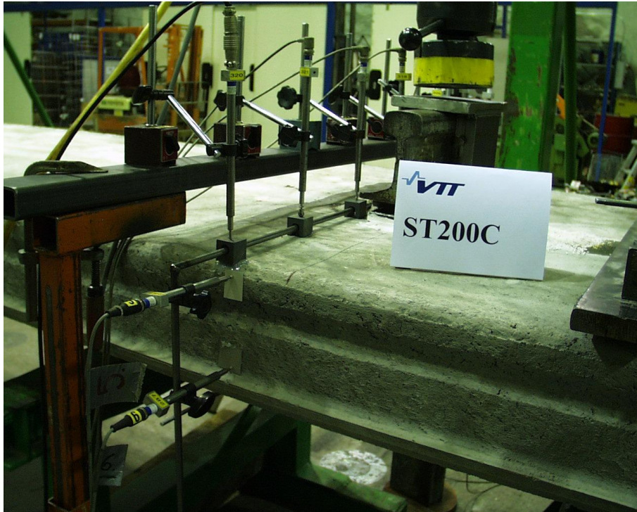
Fig. 3. ST200C. Horizontal transducers for measuring transverse shear deformation.
