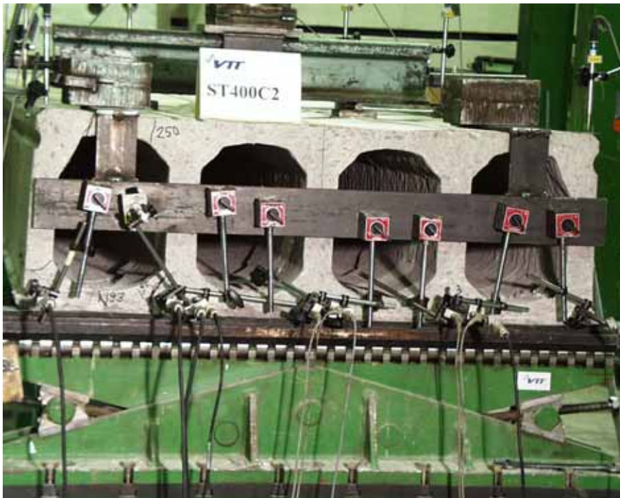
Fig. 10. ST400C2. Cracks in webs after failure.
