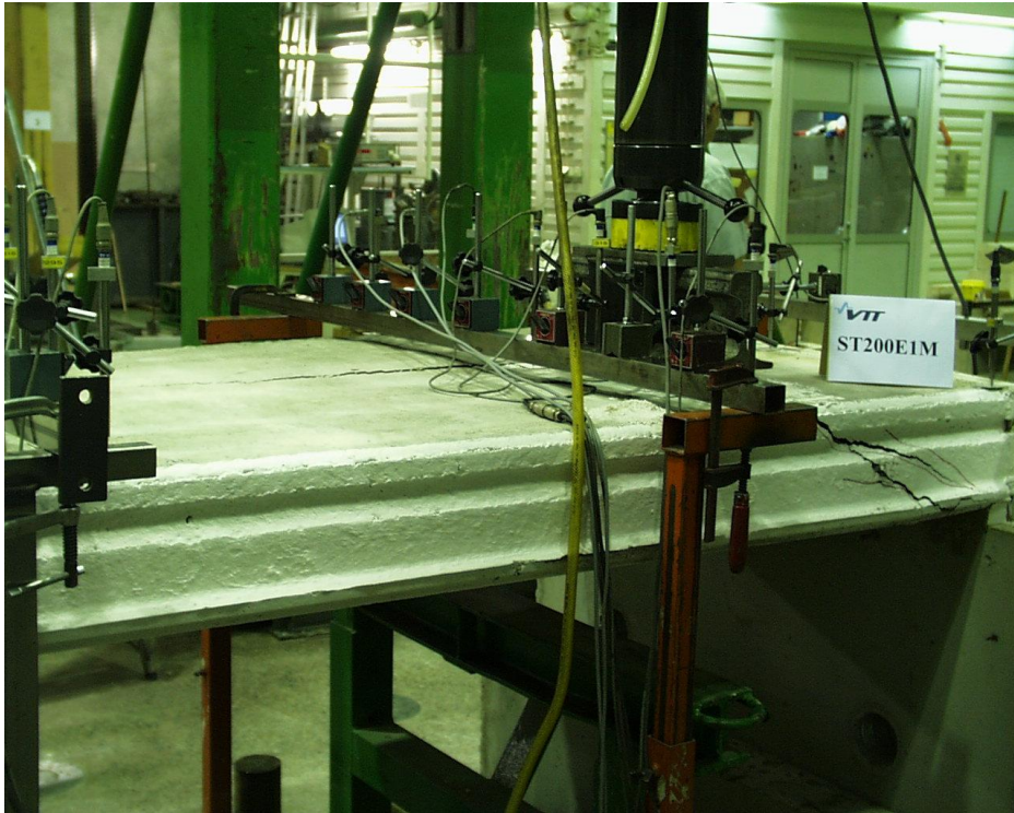
Fig. 41. ST200E1M. Cracking pattern after failure.
