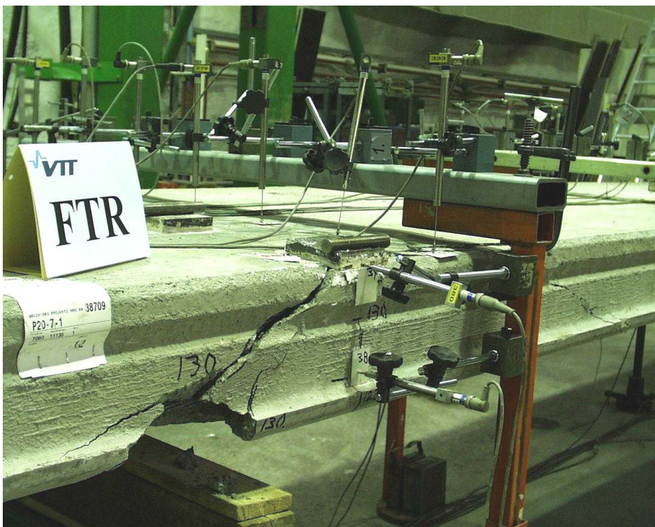
Fig. 54. ST200E2M. Cracking pattern after failure.
