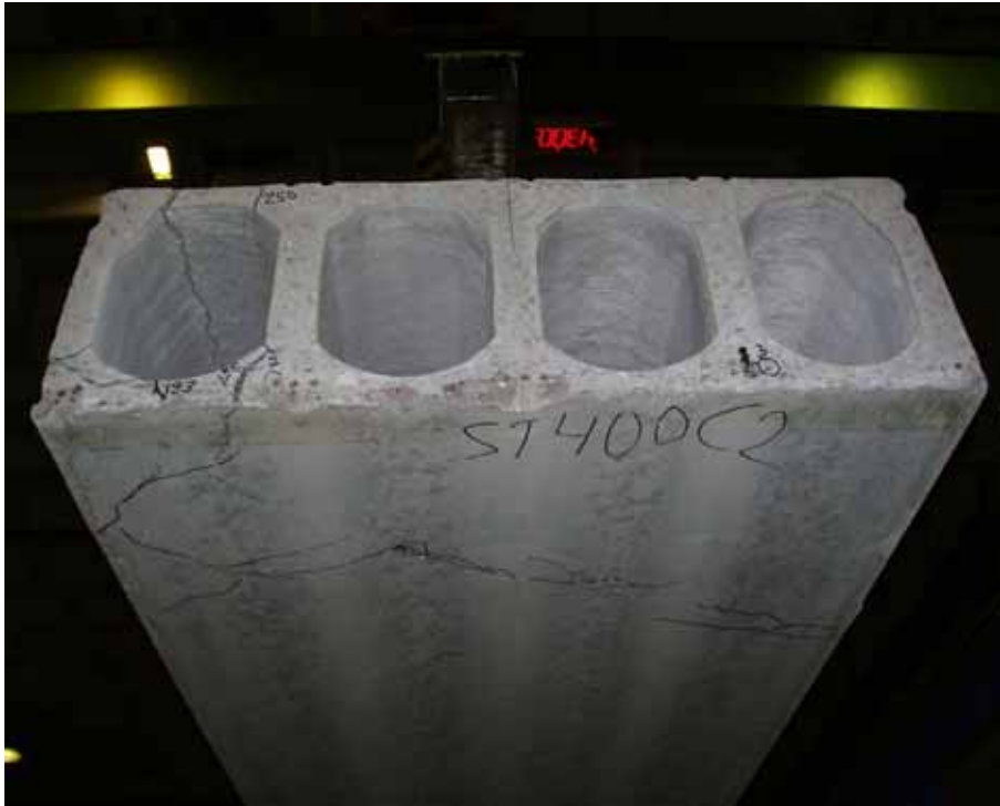
Fig. 13. ST400C2. Soffit after failure. See also Fig. 45.
