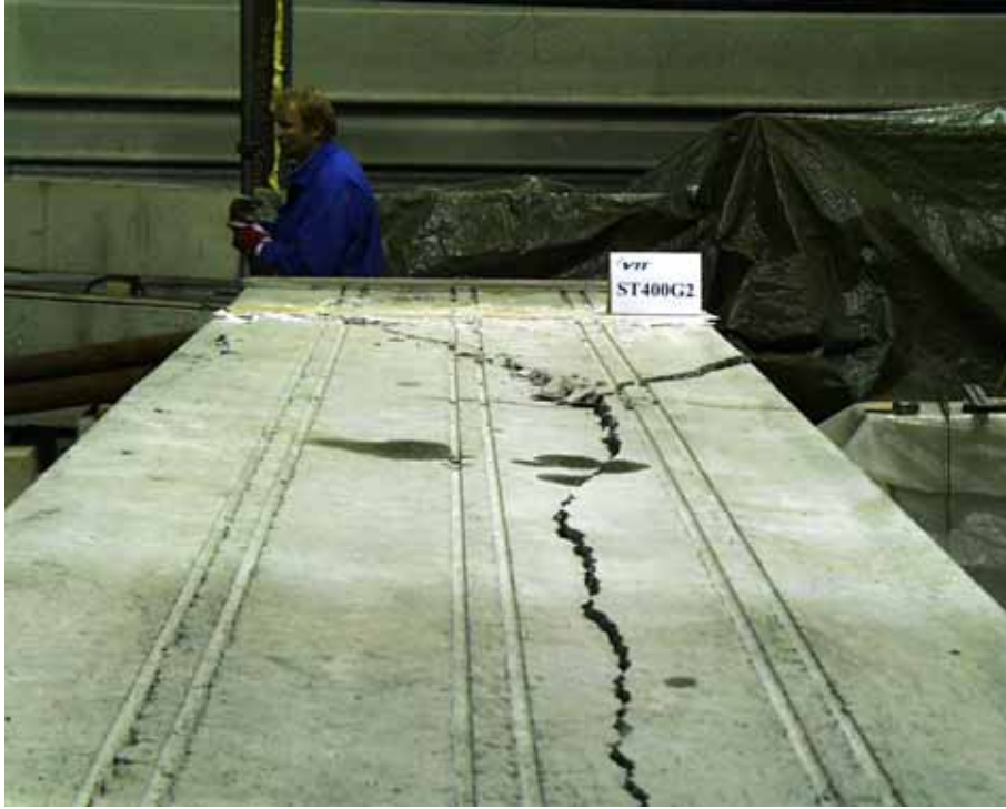
Fig. 63. ST400G2, top surface, cracks after failure.
