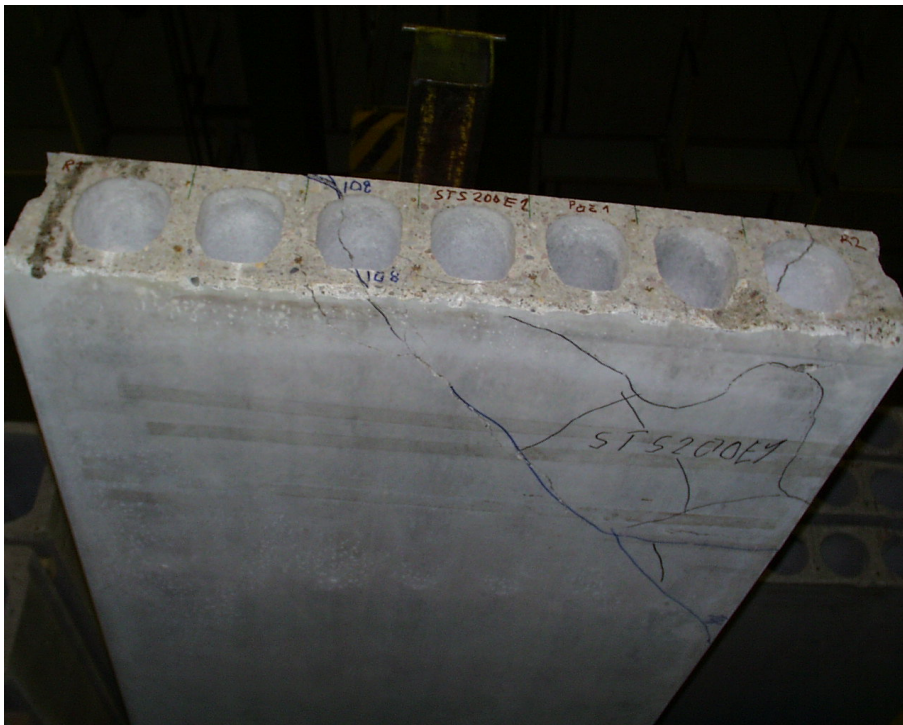
Fig. 36. STS200E1. Soffit after failure.
