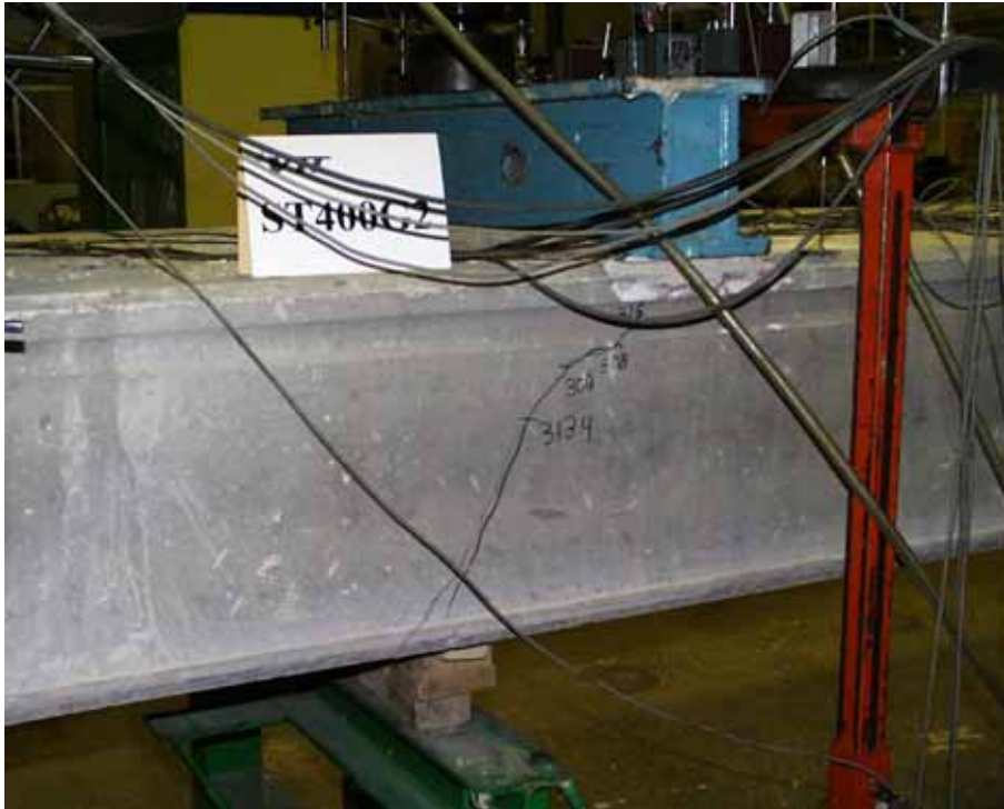
Fig. 57. ST400G2, South edge, cracks before failure.
