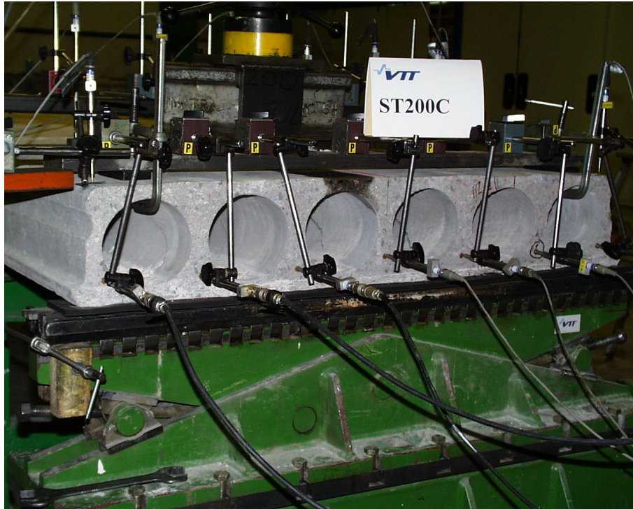
Fig. 7. ST200C. Cracks in webs after failure.
