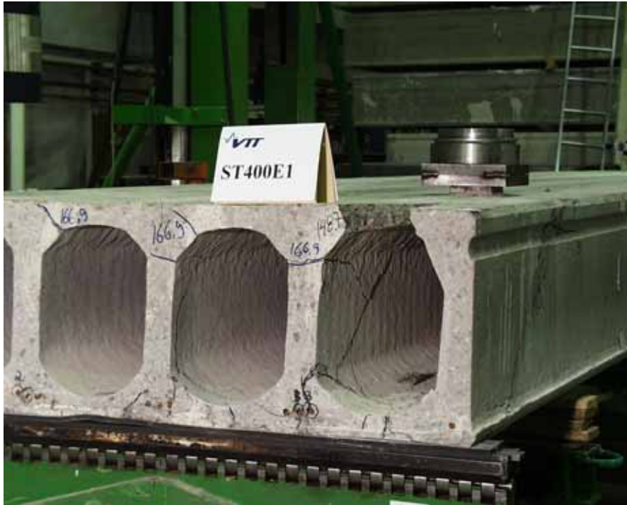
Fig. 19. ST400E1. Webs after failure.
