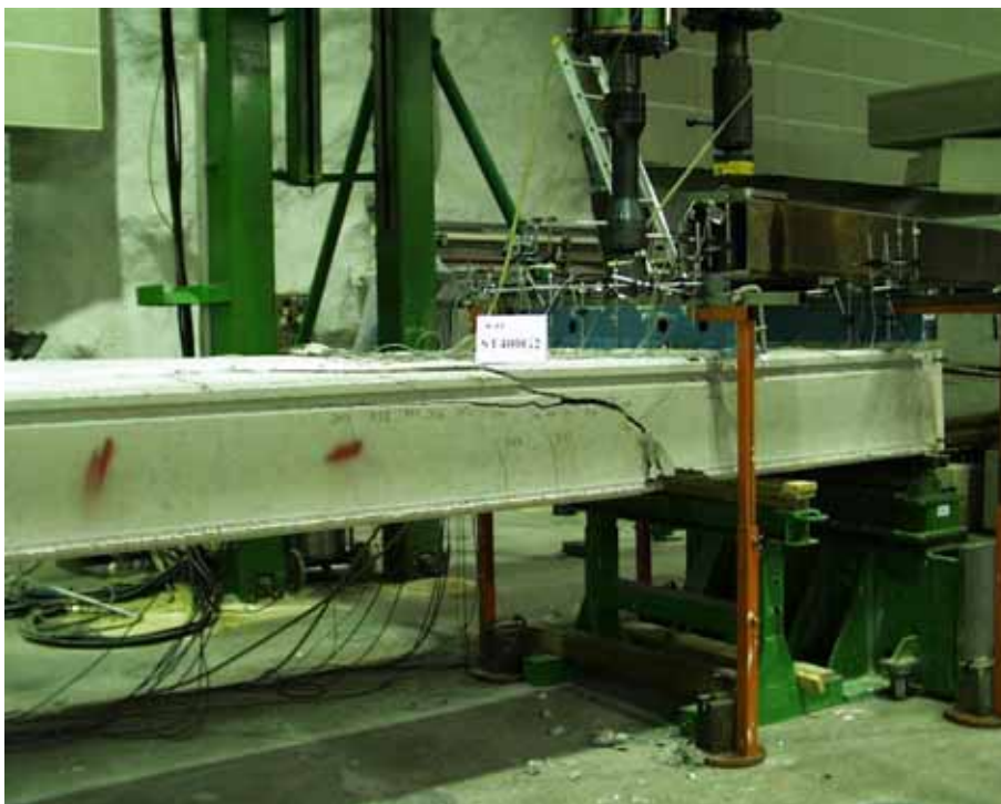
Fig. 58. ST400G2, North edge, cracks after failure.
