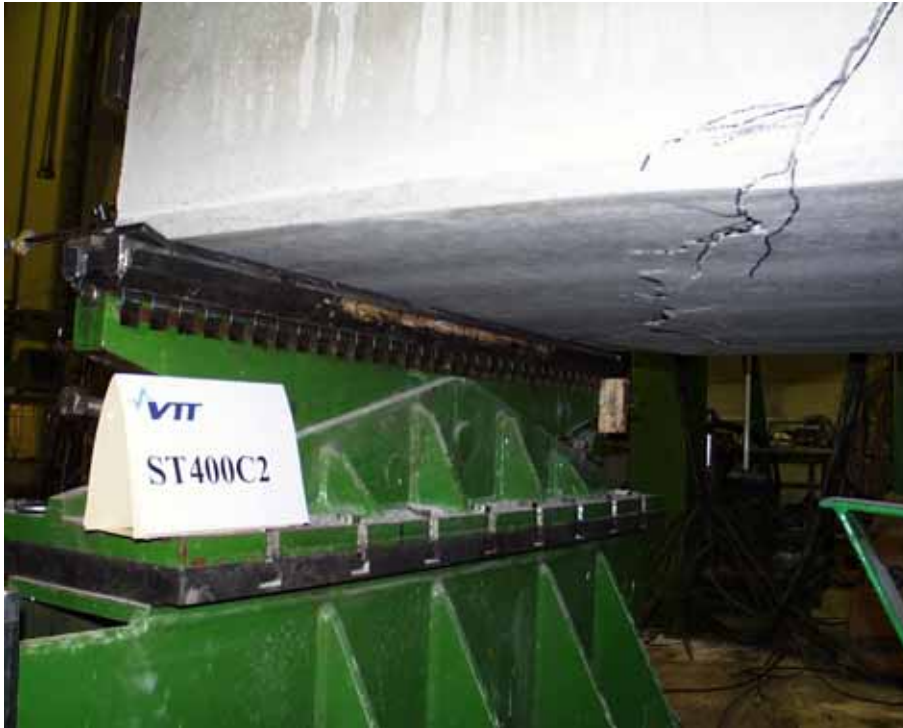
Fig. 9. ST400C2. Soffit after failure seen from the North.
