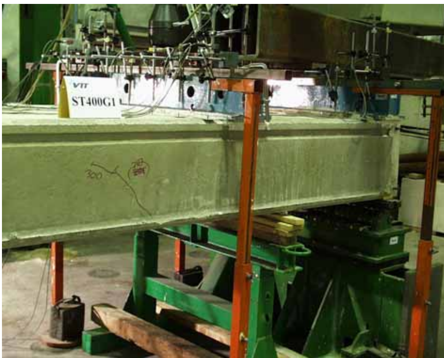
Fig. 50. ST400G1, North edge, first cracks.
