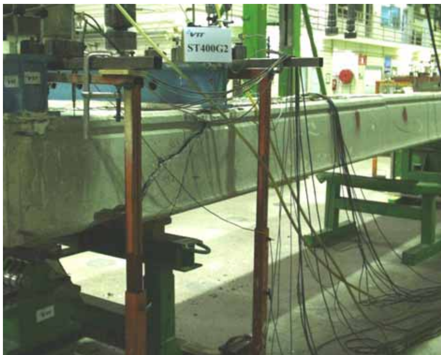
Fig. 60. ST400G2, South edge, cracks after failure.
