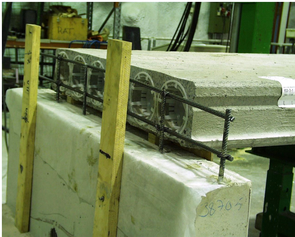
Fig. 48. ST200E2M. Arrangements at support before grouting.
