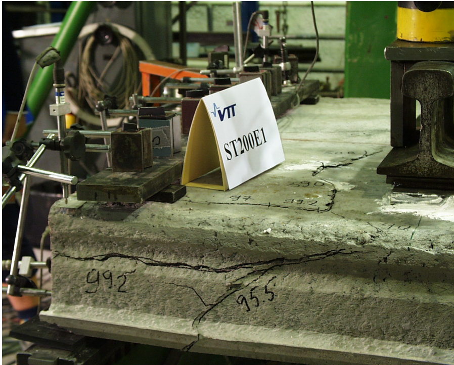
Fig. 11. ST200E1a. Cracks after failure. North edge.
