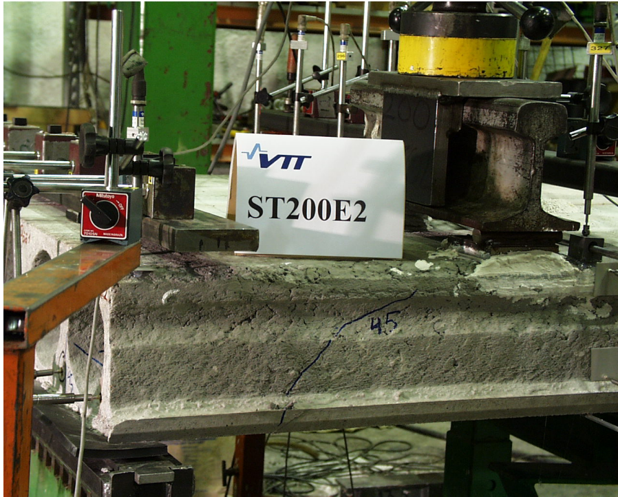
Fig. 21. ST200E2. First crack at Northern edge.
