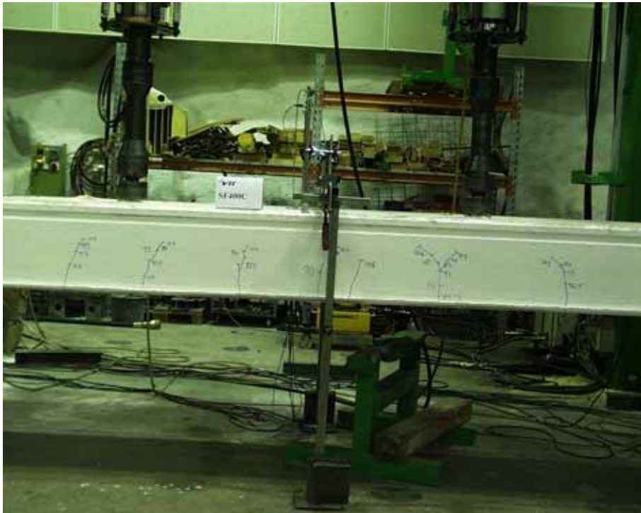
Fig. 32. SF400C. Flexural cracks in mid-span, Northern edge.
