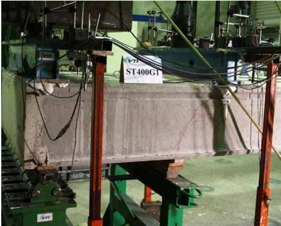
Fig. 49. ST400G1, South edge, first cracks.
