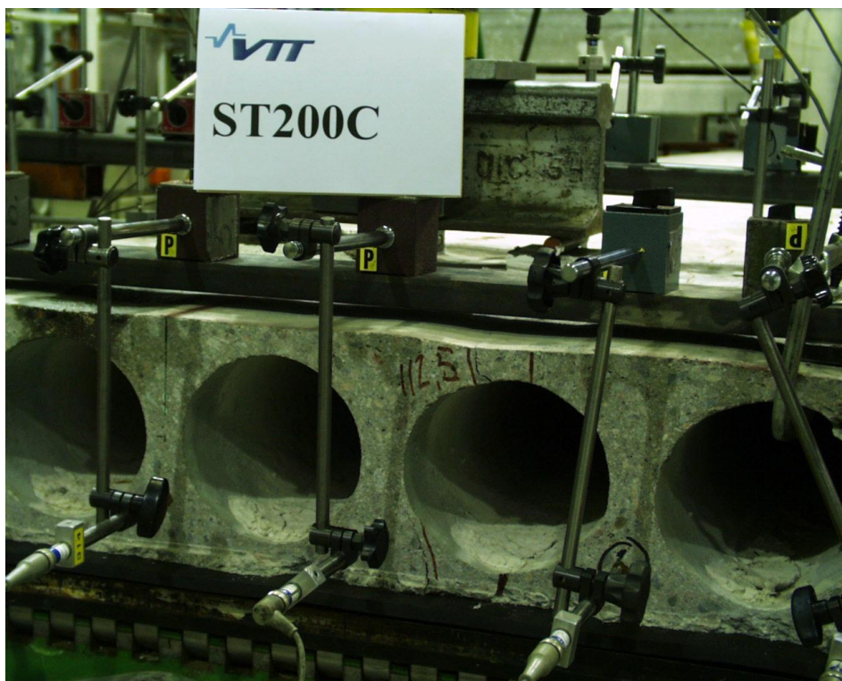
Fig. 6. ST200C. First cracks at load P = 112.5 kN.
