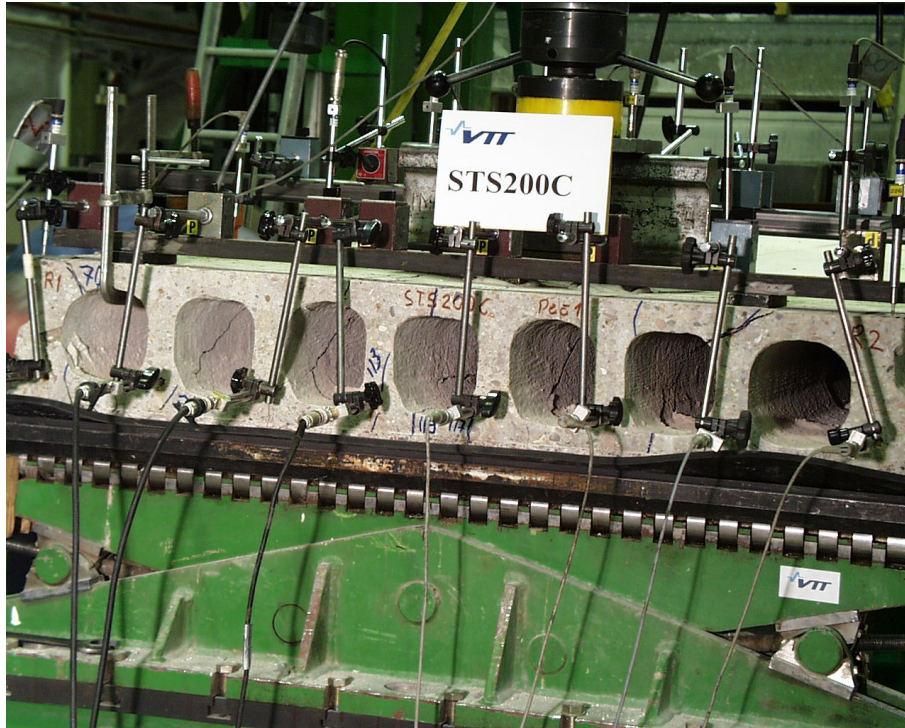
Fig. 27. STS200C. Cracking pattern in webs after failure.
