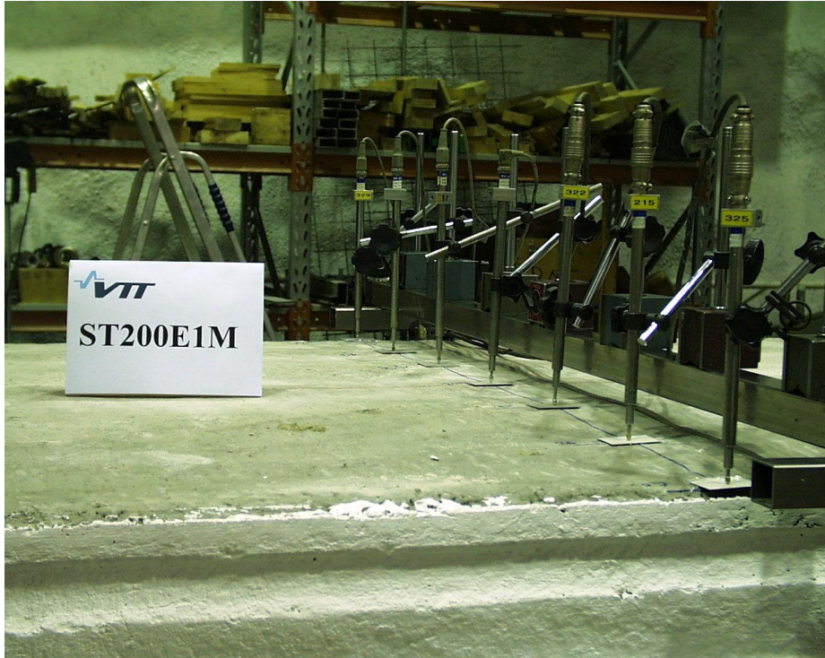
Fig. 40. ST200E1M. Measuring deflection. Note the curved top surface of the slab.
