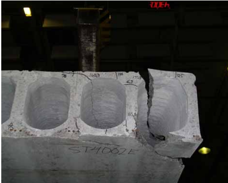
Fig. 27. ST4002E. Soffit after failure.
