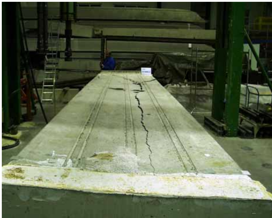
Fig. 62. ST400G2, top surface, cracks after failure.
