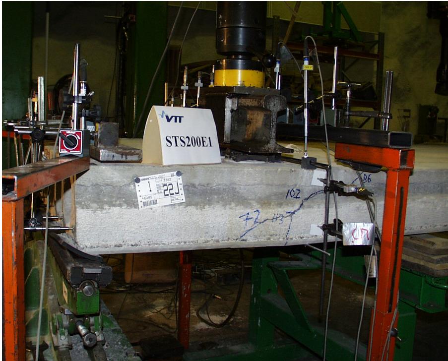
Fig. 33. STS200E1. Cracking after failure. Northern edge.
