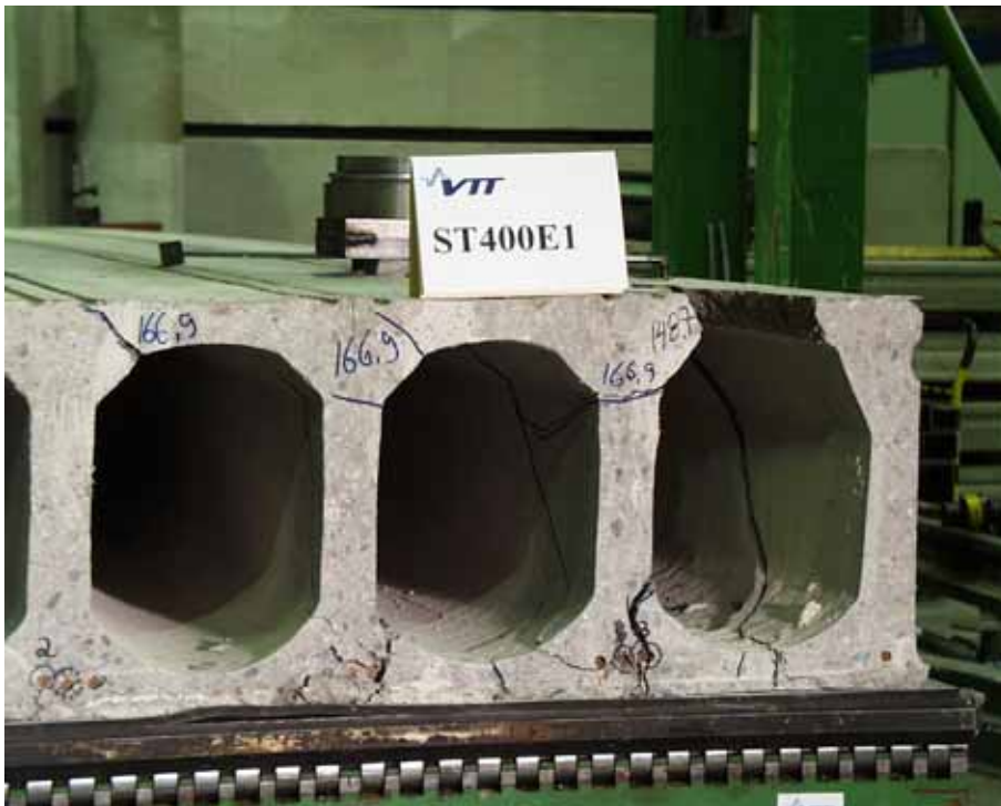
Fig. 18. ST400E1. Webs after failure.
