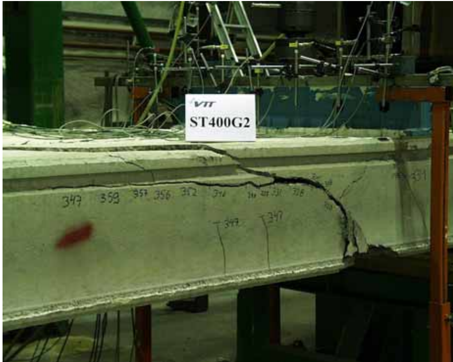
Fig. 59. ST400G2, North edge, detail of failure cracks.
