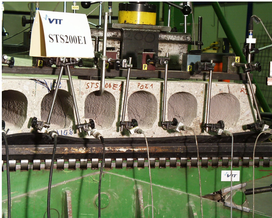
Fig. 32. STS200E1. Cracking pattern in webs after failure.
