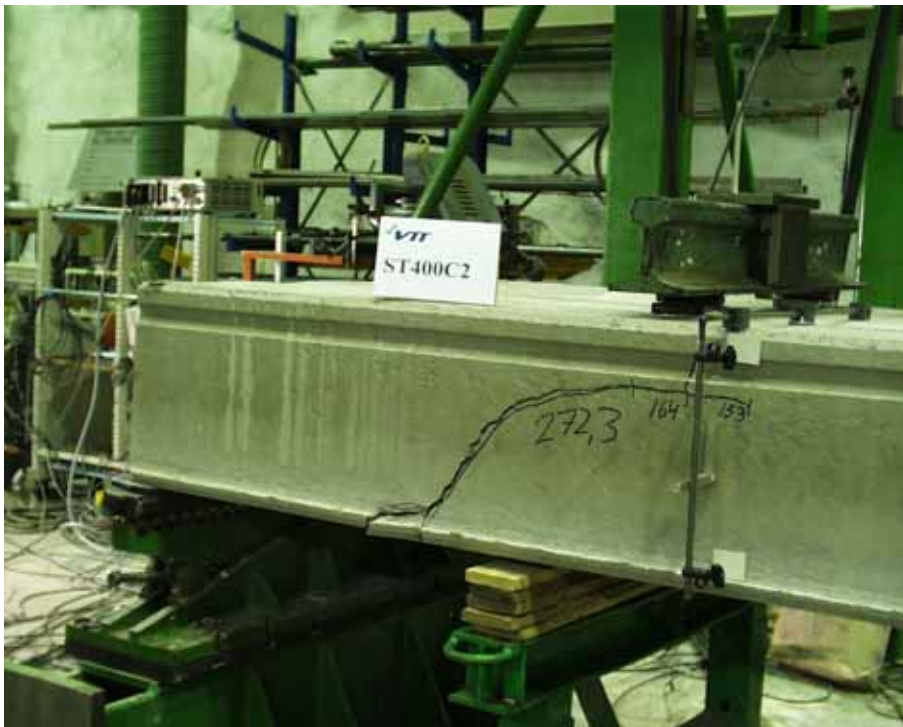
Fig. 12. ST400C2. Northern edge after failure.
