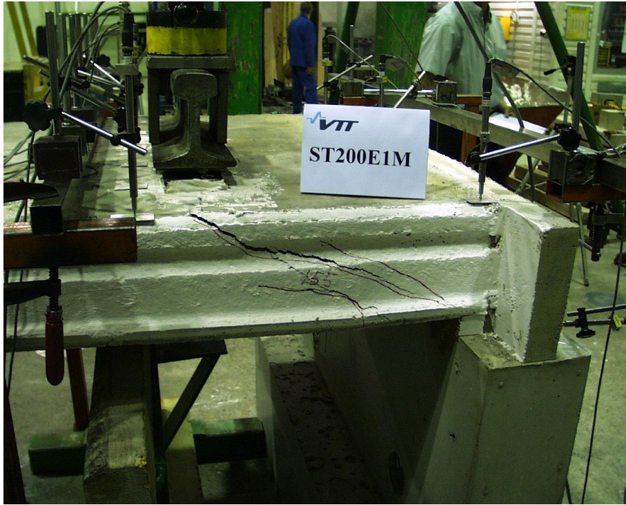
Fig. 43. ST200E1M. Cracking pattern between load and support.
