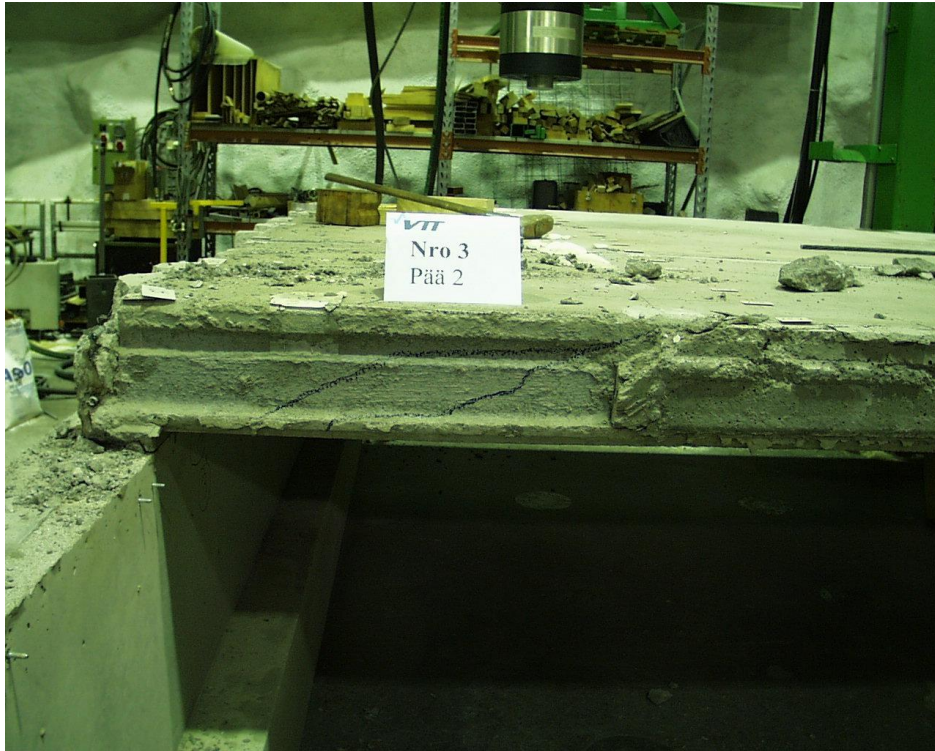
Fig. 39. FT200:11. End 2 of slab 3 after removing slab 4.
