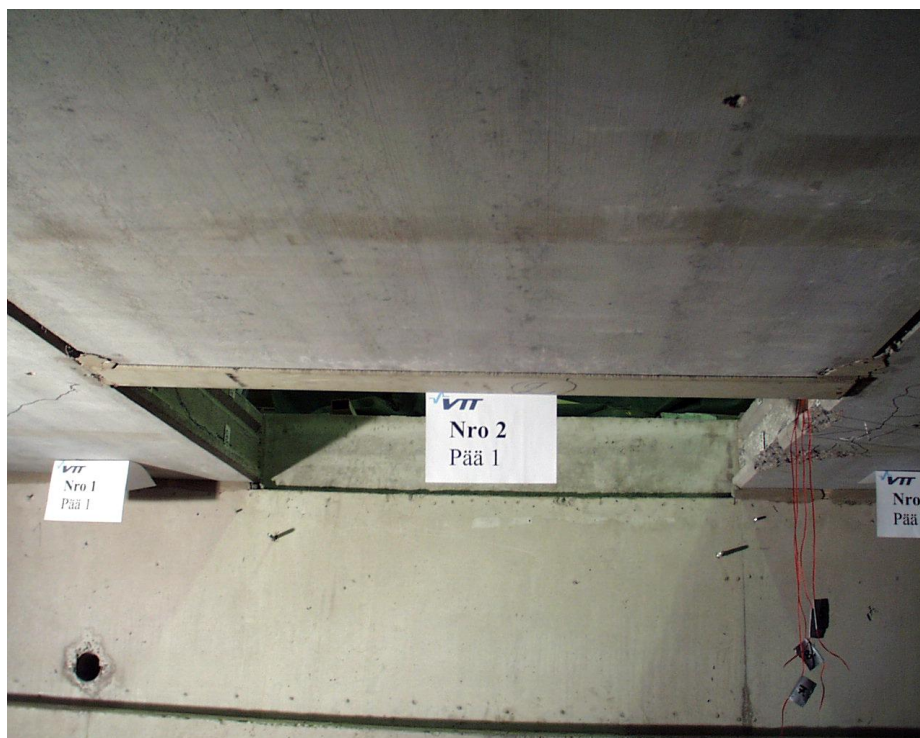
Fig. 30. FT200:12. Virtually uncracked soffit of slab 2 after failure.
