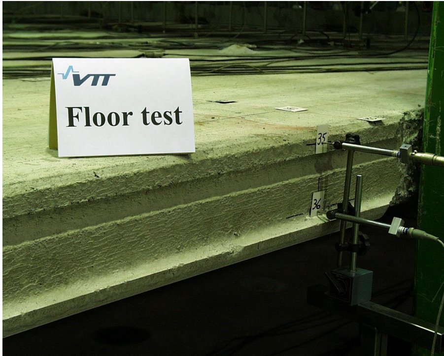
Fig. 9. Transducers for measuring horizontal displacement of outer edges of floor.
