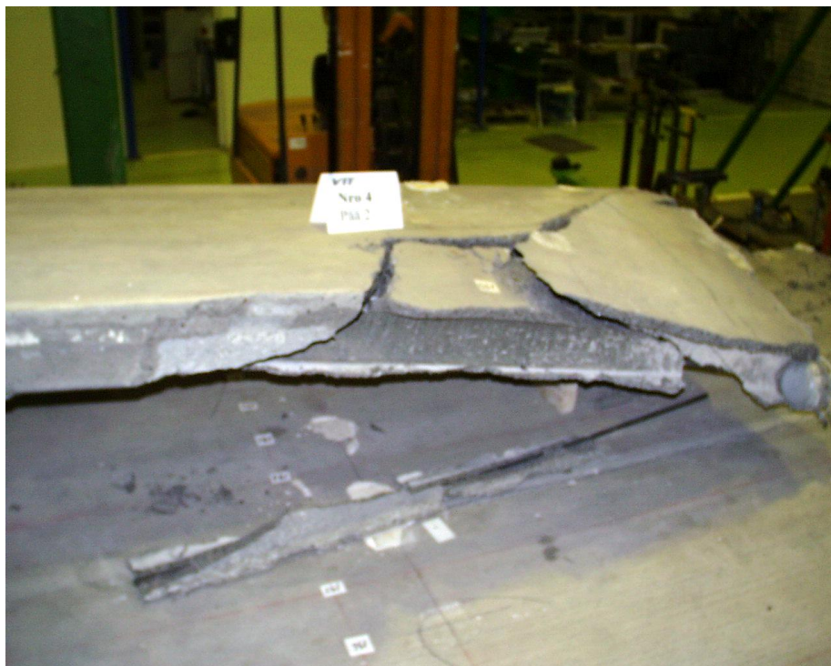
Fig. 36. FT200:11. End 2 of slab 4 after demolishing of floor.
