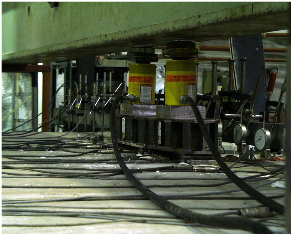
Fig. 16. FT200:12. Loading arrangements.
