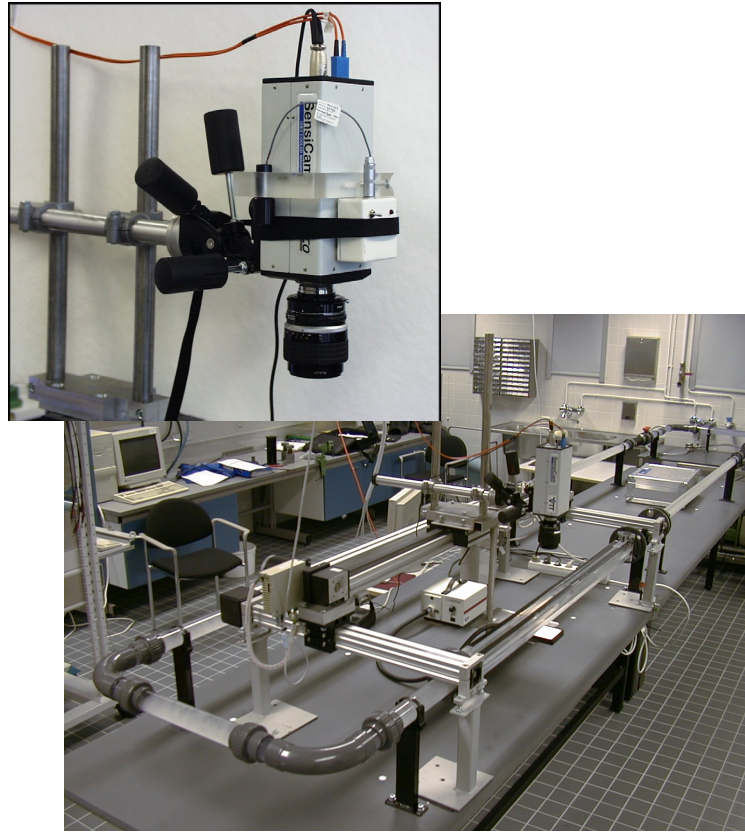
Figure 1. PCO SensiCam mounted on a flow line at VTT flow research laboratory.
