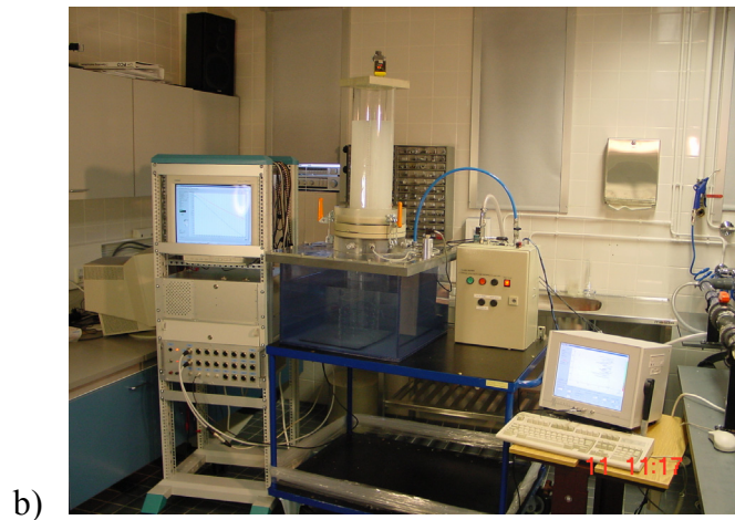
Figure 1 a) Schematic illustration and b) laboratory set-up of the filtration device based on pulsed ultrasound-Doppler anemometry.
