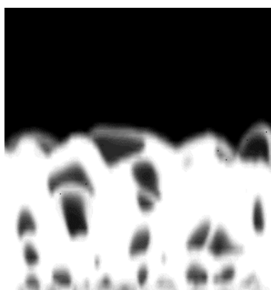
Figure 10. Spontaneous bubbling simulated with drag model 9 plotted using a linear color scale.
