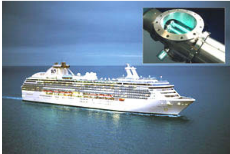
Figure 7. Cruise ship Coral Princess, which is equipped with a combination of filter and UV disinfection as a ballast water treatment method (Berson, 2004).
