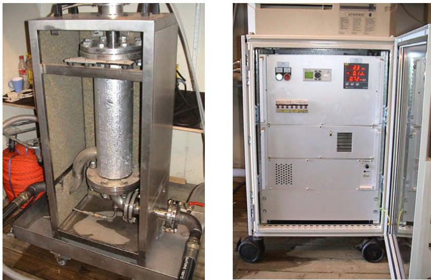
Figure 4. The 4 kW US and power control unit during the onshore test trials.
