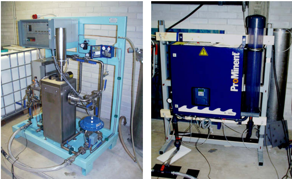
Figure 3. Left: Ultraviolet light and ultrasound devices mounted in the same aggregate. The US transducer is mounted inside the stainless steel box. Right: The ozone device rig during the Espoo trials.
