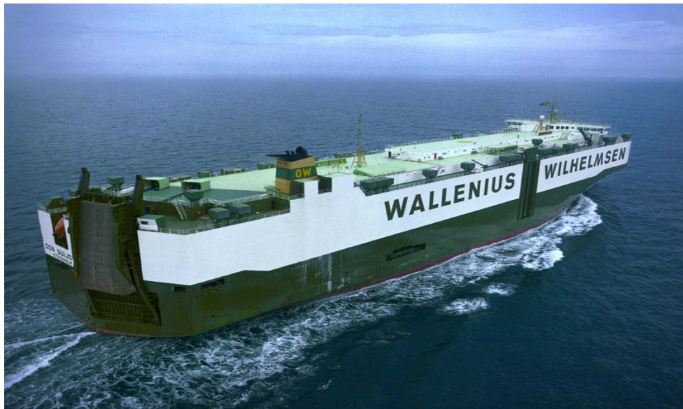
Figure 9. M/V Don Quijote , 14,800 dwt pure car and truck carrier (Wallenius Lines, 2005).
